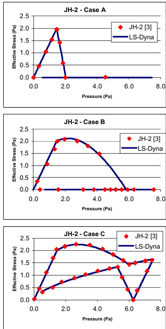
**Figure 3** Stress versus pressure histories for single element validation cases
