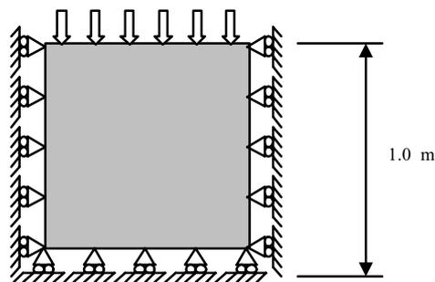
**Figure 2** Test case boundary conditions
