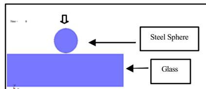
**Figure 4** Sample calculation finite element model
