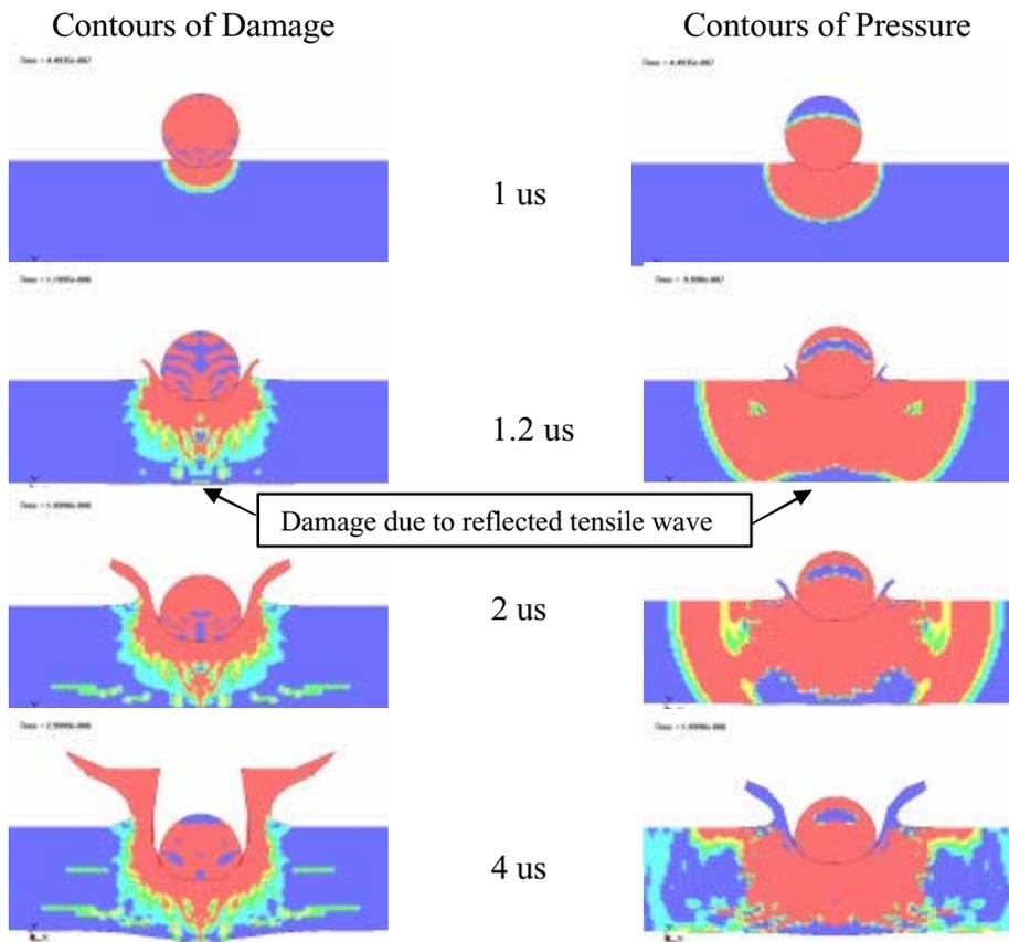
**Figure 5** Sample calculation finite element model
