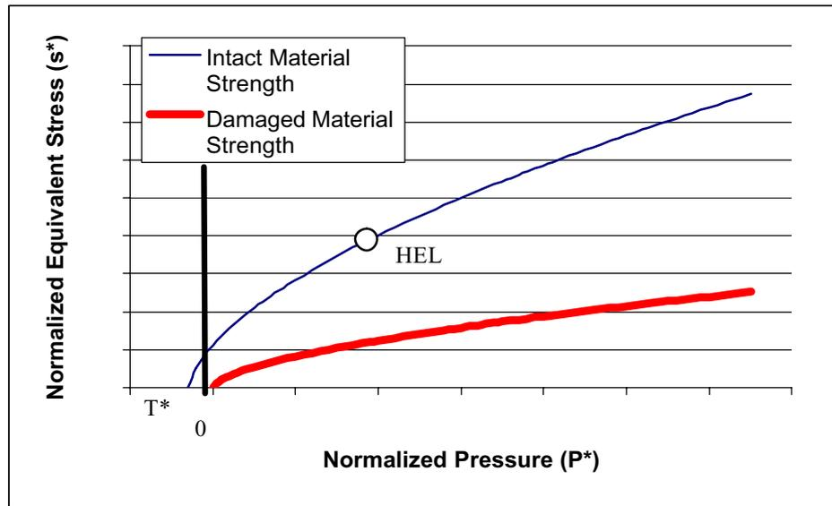
**Figure 1** Strength versus pressure for intact (undamaged) and damaged material
