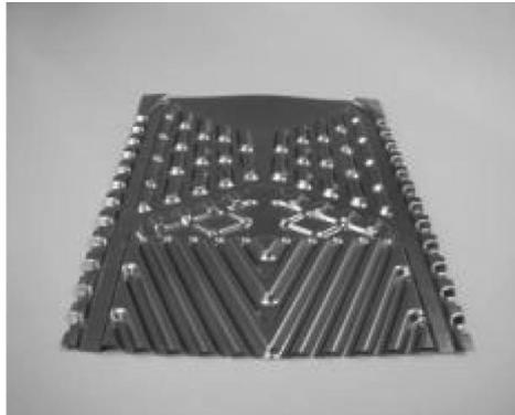
**Figure 1: Special heat exchanger plate in stainless steel**
