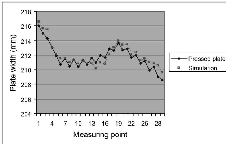
**Figure 10: Comparison of outer dimension for pressed heat exchanger plate and simulated heat exchanger plate.**
