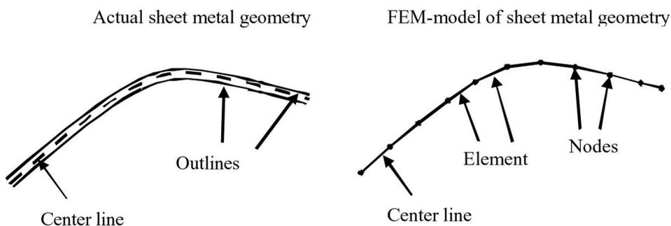
**Figure 4: Actual sheet metal geometry and FEM-model of the same**
