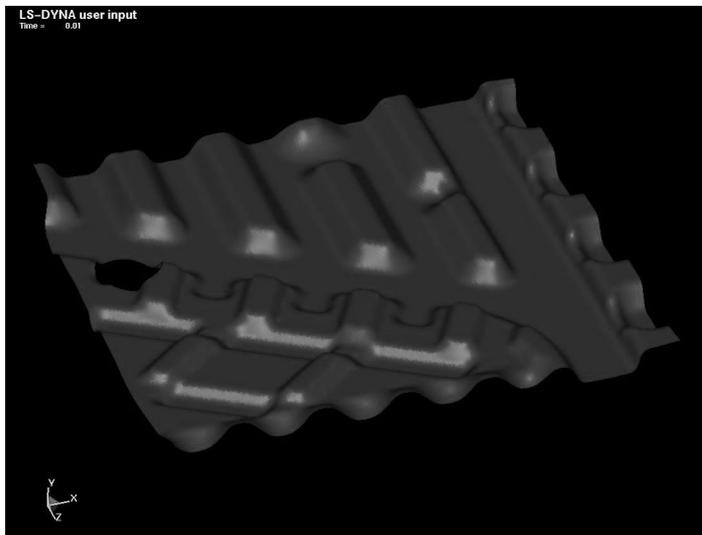
**Figure 3: Section of simulated test heat exchanger plate created as input for different parallel simulations**
