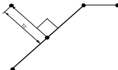
**Figure 5: A new node is created at half thickness from original node perpendicular to centre line**
