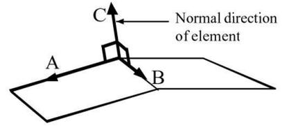
**Figure 7: The normal to a element C is calculated from edges A and B**
