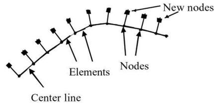
**Figure 6: New nodes are creating the outer surface**
