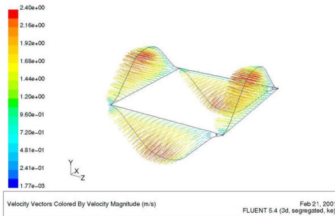
**Figure 11: Result from simulation of computational fluid dynamics performed on forming simulated section of a heat exchanger plate**
