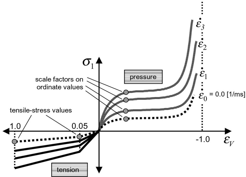
**Figure 6: Definition of the design variables: 4 ordinate scale factors + 2 tensile stress values.**
