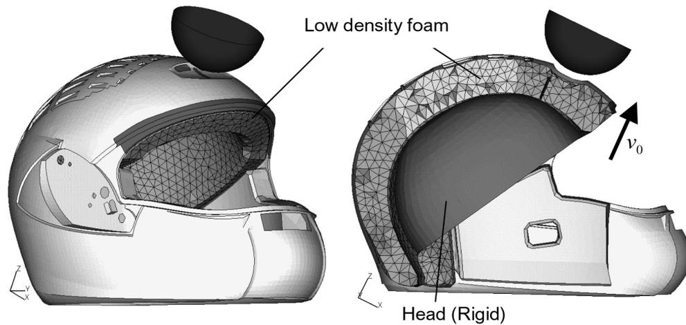
Figure 3: Impact of a helmet on a rigid hemisphere.
