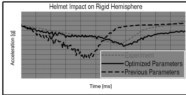
**Figure 9: Simulation and experimental data of the helmet drop test.**
