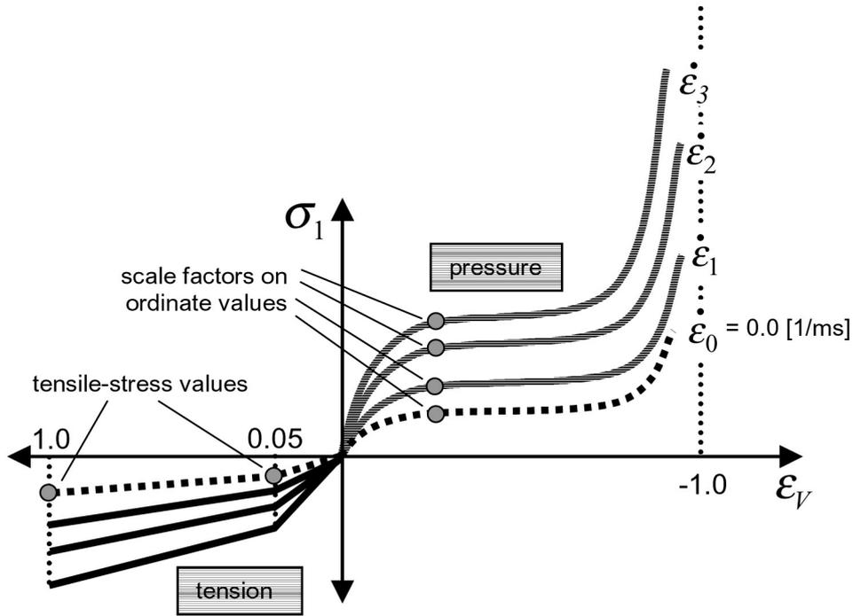
**Figure 6: Definition of the design variables: 4 ordinate scale factors + 2 tensile stress values.**
