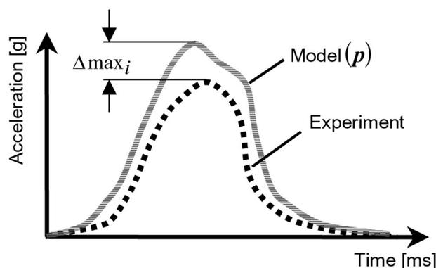
Figure 5: The target value to be minimized within the optimization.
