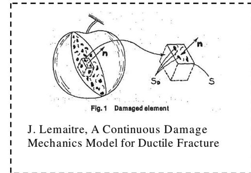
Fig.1 Damaged element
