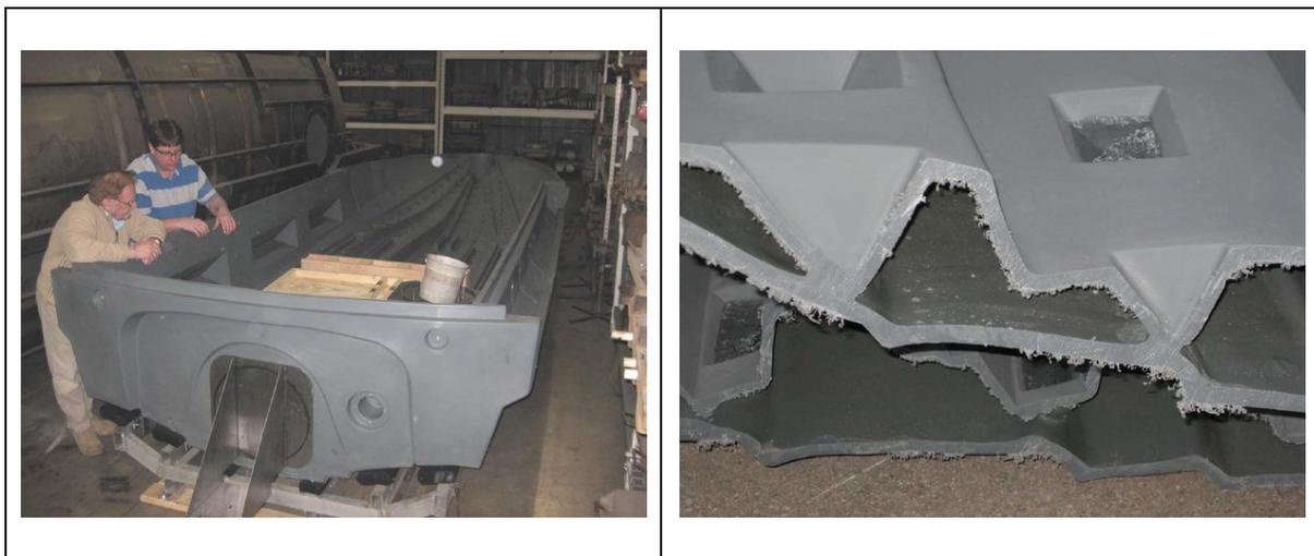
Figure 3: First molded hull and cut-away showing the patented "kiss-off" connection
