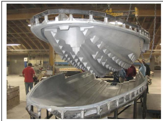
Figure 2: 7-meter boat molding tools
