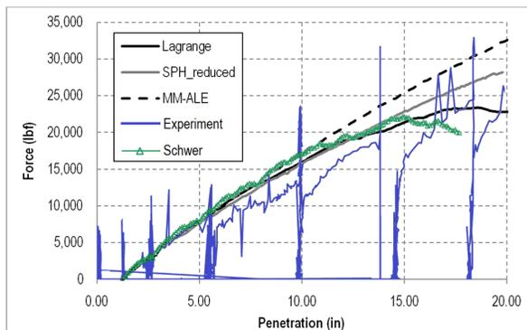
Figure 15: Comparison of the measured force versus displacement [1]
