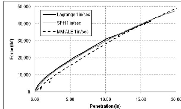
Figure 10: Force as a function of loading pad penetration for three models: Lagrangian, SPH\_reduced and MM-ALE
