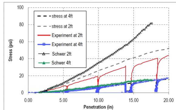
Figure 16: Comparison of the measured stresses under the pad versus displacement [1]
