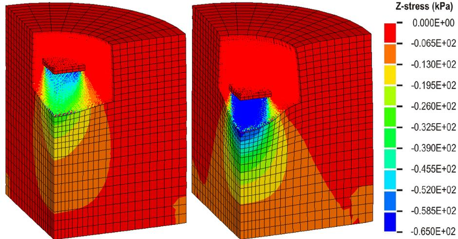
Figure 8: Deformations and Z stresses in SPH model
