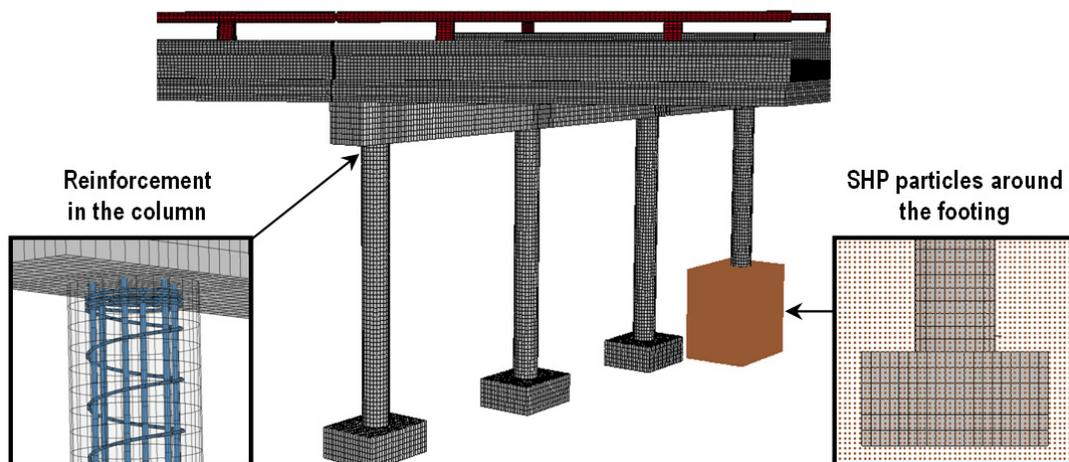
Figure 2: FE model of Oat Ditch Bridge
