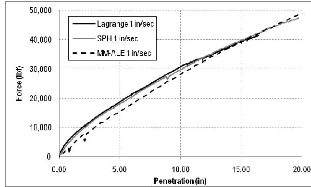
Figure 10: Force as a function of loading pad penetration for three models:
