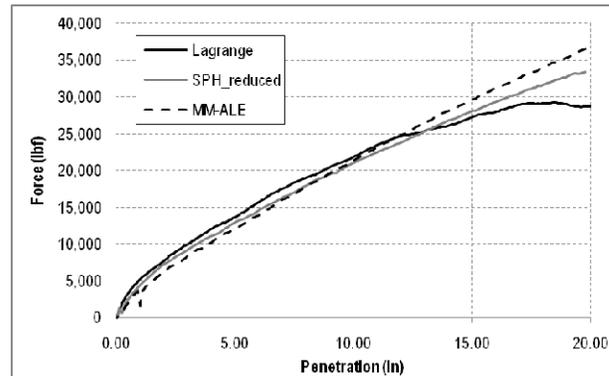
Figure 14: Force as a function of loading pad penetration for soil with low density
