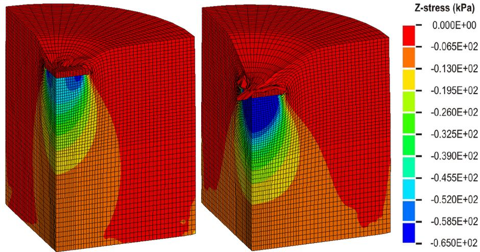
Figure 7: Deformations and Z stresses in Lagrange model
