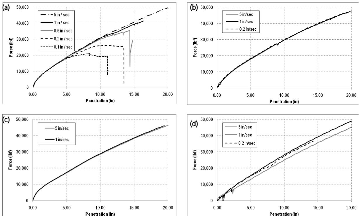
Figure 13: Force as a function of loading pad penetration for models:
