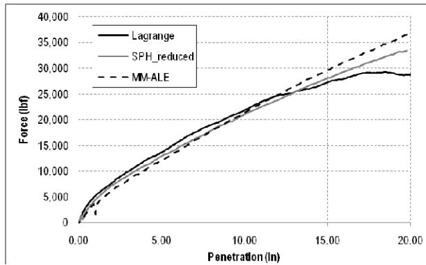
Figure 14: Force as a function of loading pad penetration for soil with low density
