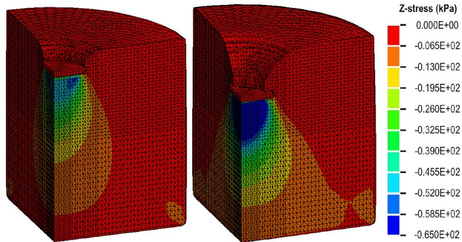
Figure 9: Deformations and Z stresses in MM-ALE model
