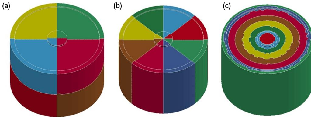
Figure 5: Decomposition methods (a) default, (b) wedge type, (c) cylindrical
