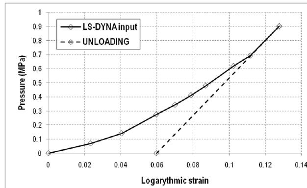
Figure 3: Hydrostatic compression data for soil material [1]
