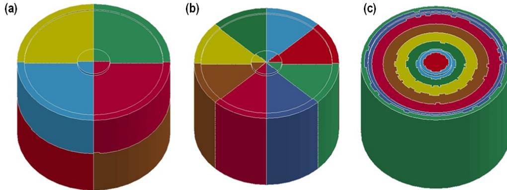
Figure 5: Decomposition methods (a) default, (b) wedge type, (c) cylindrical
