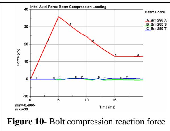
**Figure 10-** Bolt compression reaction force
