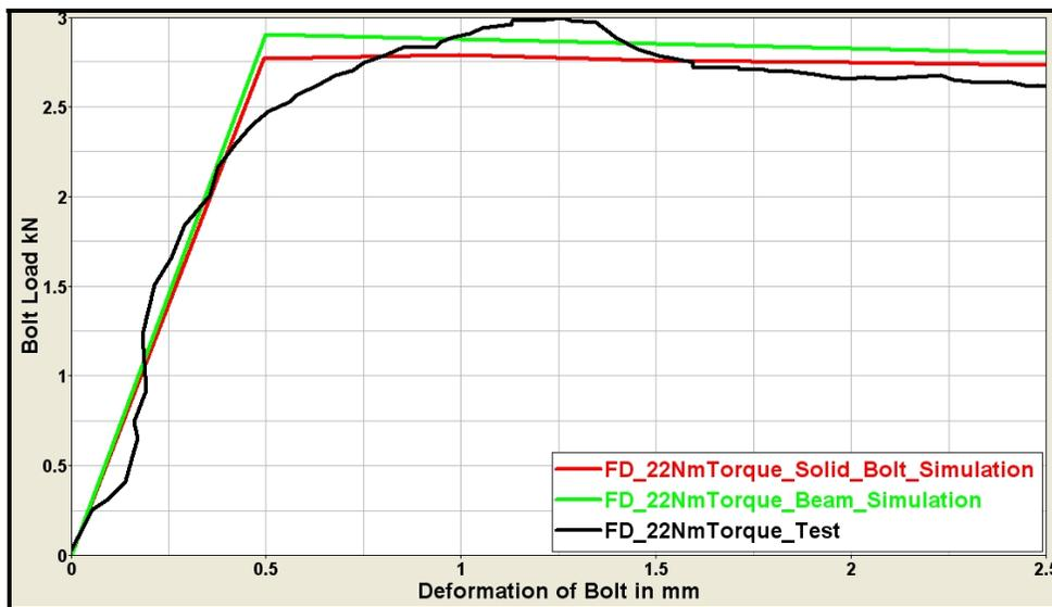
Figure 15 - Forces Vs displacement tapped from physical test and FEM model for sliding test
