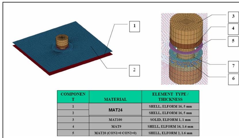
**Figure 3-** Hex solid element Bolt with appropriate contact
