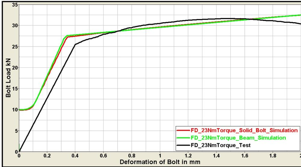
Figure 14 - Forces Vs displacement tapped from physical test and FEM model for tension test
