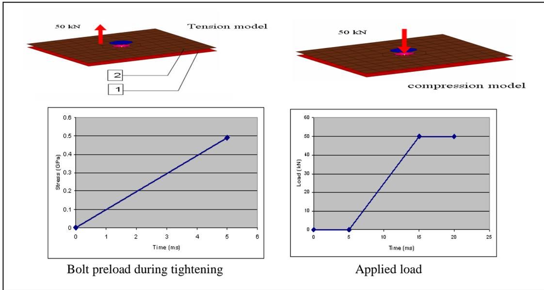
**Figure 8** –Test set up for bolt tension/compression test with applied pre-load and prescribed force
