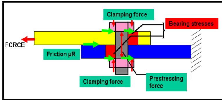
Figure 1- Bolt joint with forces and stresses
