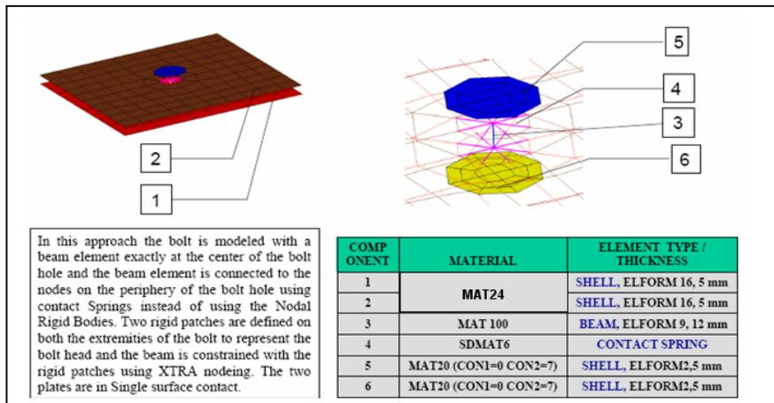
Figure 2-1D Beam with discrete spring
