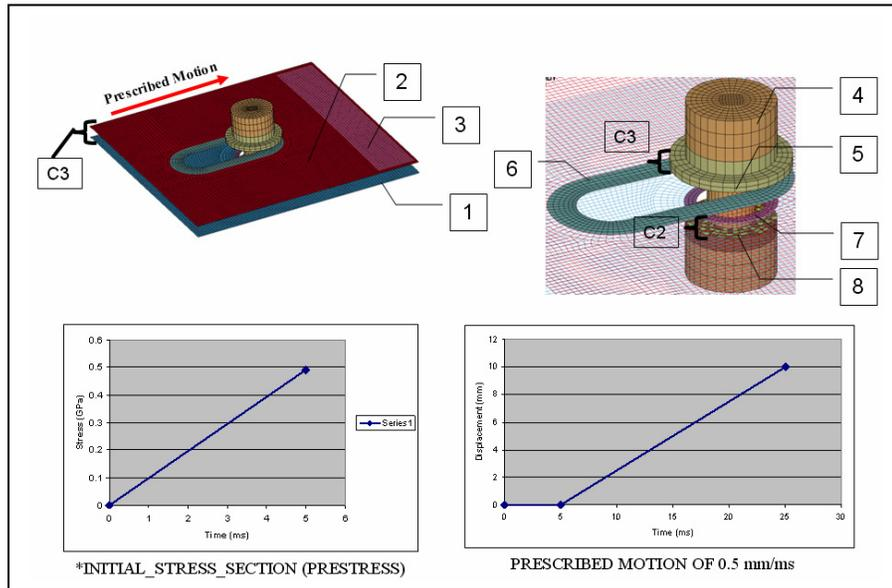
**Figure 11** –Test set up for sliding test with applied pre-load and prescribed motion
