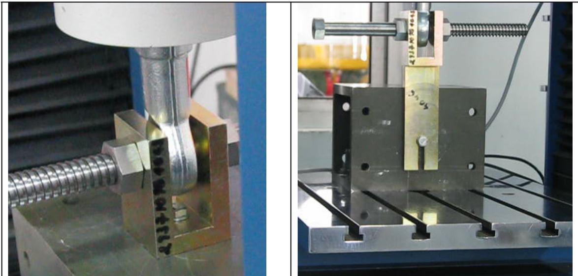
**Figure 13** : Tension and sliding test set up for bolted joint testing
