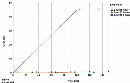
Figure 7 - Bolt forces reaction forces
