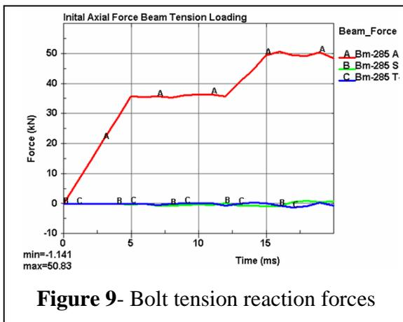
**Figure 9-** Bolt tension reaction forces
