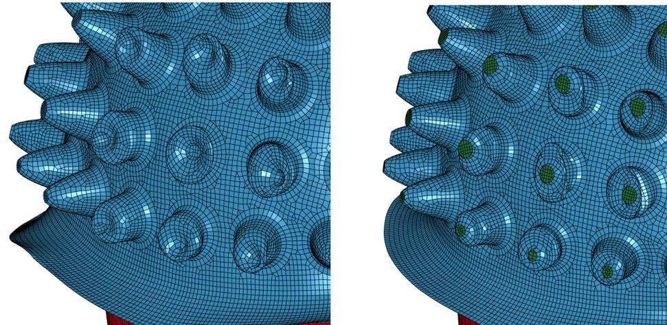
Fig. 12 Comparison between deformed shape for uncoupled and coupled shell-liner configuration for 0.85 mm liner thickness.
