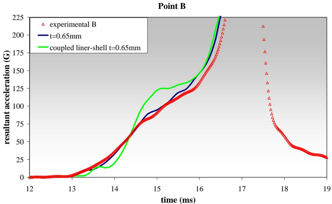
Fig. 10 Numerical comparison between uncoupled and coupled shell-liner configuration for 0.65 mm liner thickness.
