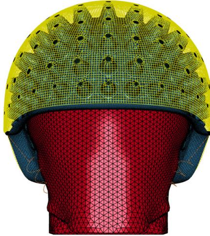
Fig. 9 FE modeling of the coupled liner-shell helmet.
