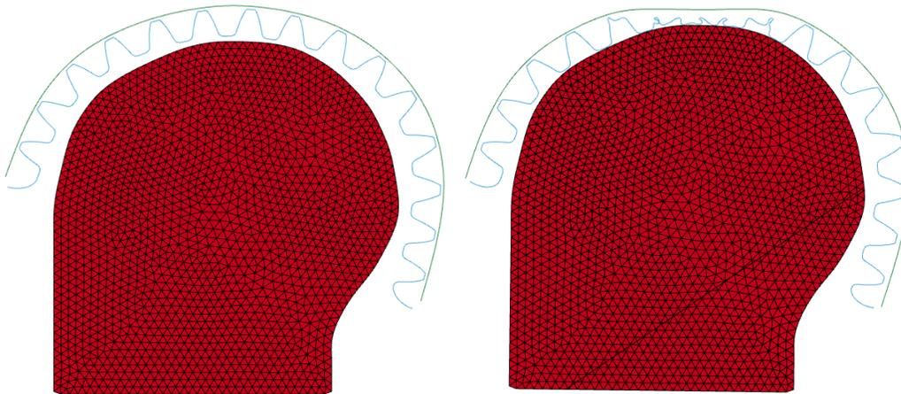
Fig. 6 Cross section of the helmet at initial time step (left) and after the impact (right).
