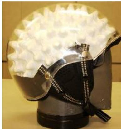
Fig. 2 Ski helmet prototype on the headform.
