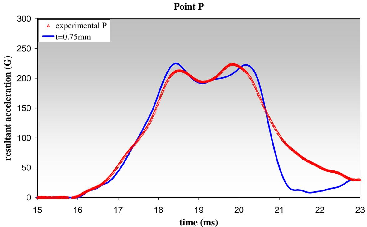
Fig. 7 Experimental versus numerical acceleration at the crown.
