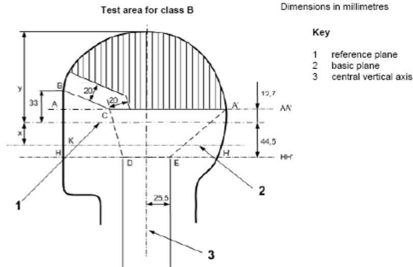
Fig. 1 Test area (dashed) of EN1077 class B.
