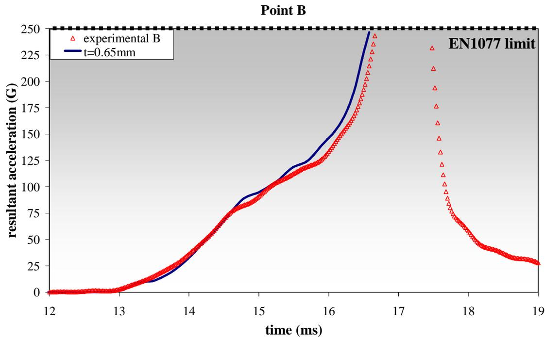
Fig. 8 Experimental versus numerical acceleration at the front.
