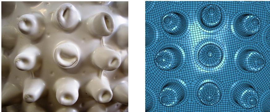
Fig. 5 Experimental and numerical deformed shape at the crown.
