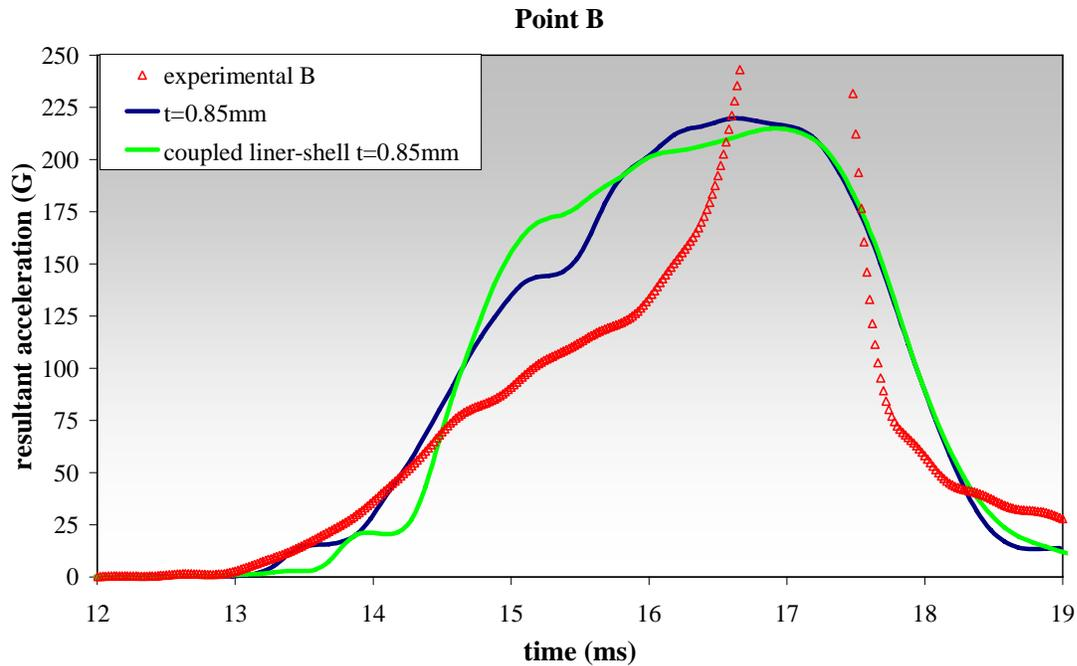
Fig. 11 Numerical comparison between uncoupled and coupled shell-liner configuration for 0.85 mm liner thickness.
