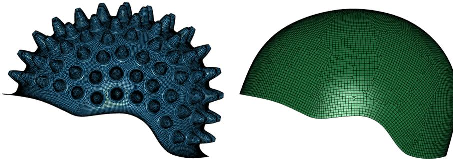
Fig. 3 Discretized geometry of ABS liner and PC shell.
