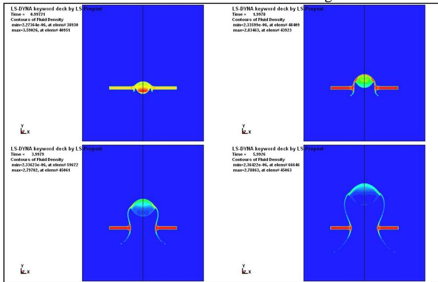
Figure 2 : Views of HVI at various steps of simulation
