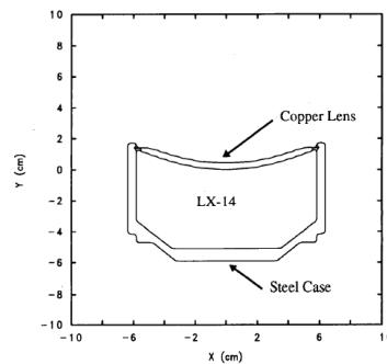
Figure 9 : Initial EFP configuration
