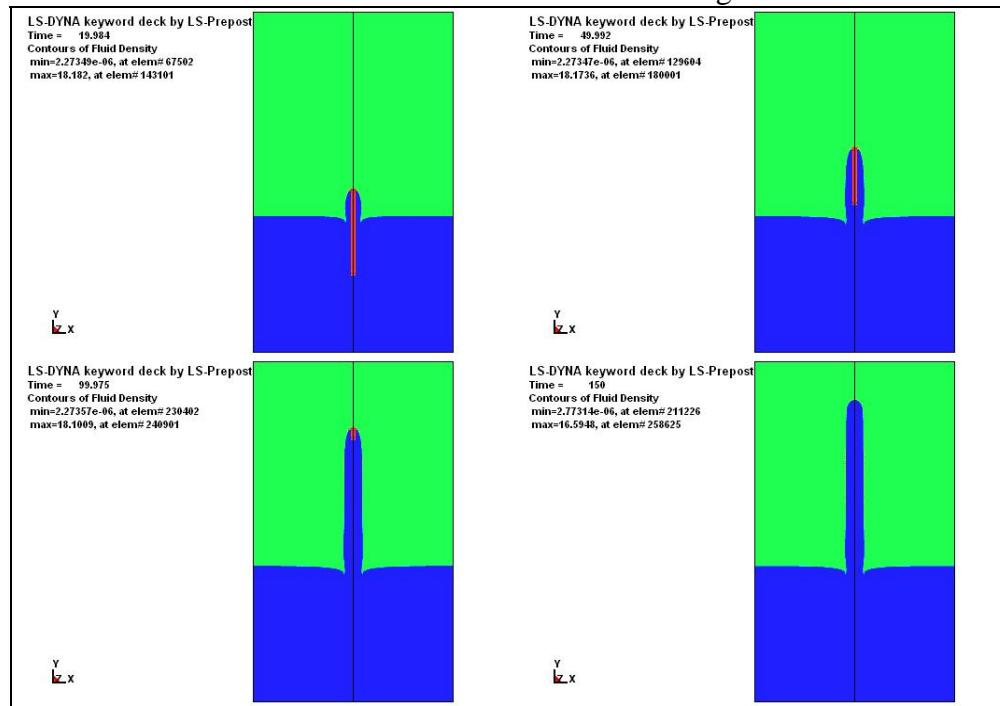
**Figure 5 : Views of Long rod penetration at various steps of simulation**
