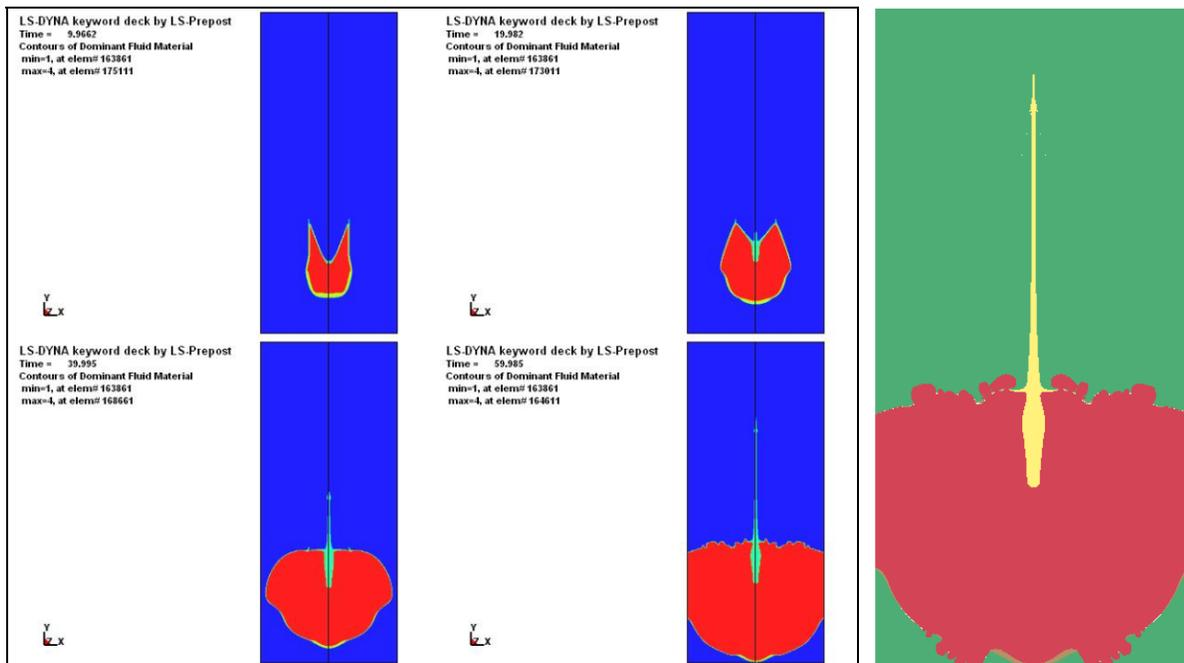
Figure 15 : Views of Shaped Charge Jet at various steps of simulation
