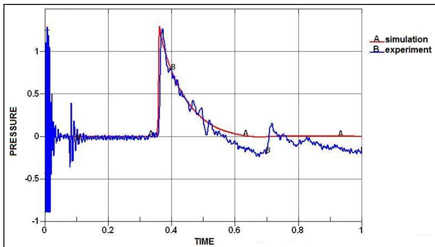
**Figure 17 : Result example given by LS-DYNA on Air blast study**
