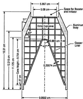
Figure 13 : Initial configuration of Shaped Charge
