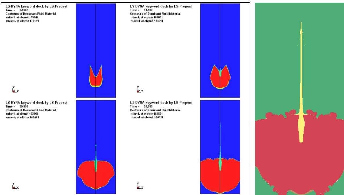
Figure 15 : Views of Shaped Charge Jet at various steps of simulation
