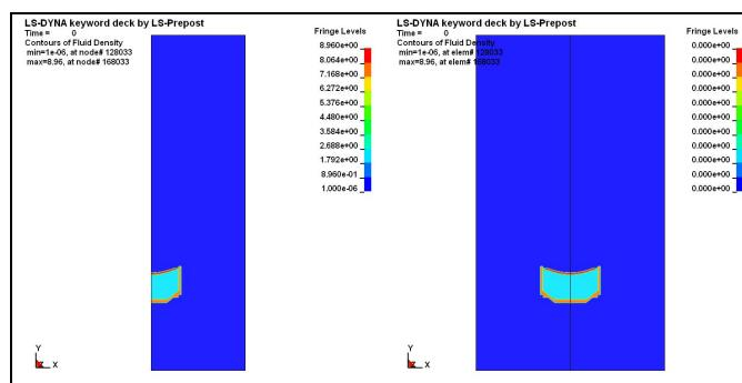
Figure 10 : Initial configuration of LS-DYNA model
