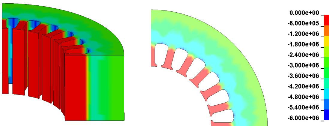
Figure8. Compressive Stress Distribution (Pa)
