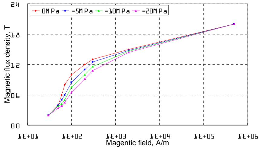
Figure3. Stress Dependent BH Curve (stator core)
