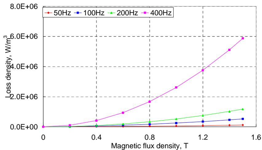
Figure7(b). Core-Loss of the Stator Core (stress: -10 MPa)
