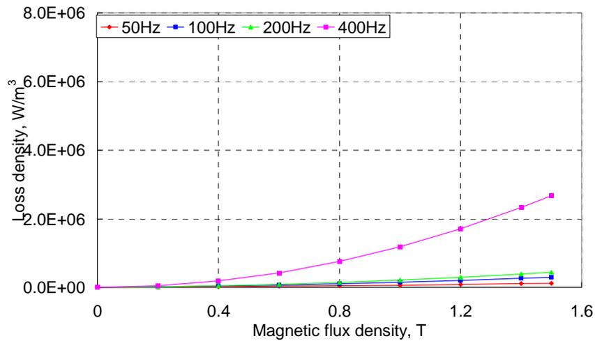
Figure7(a). Core-Loss of the Stator Core (stress: 0 MPa)
