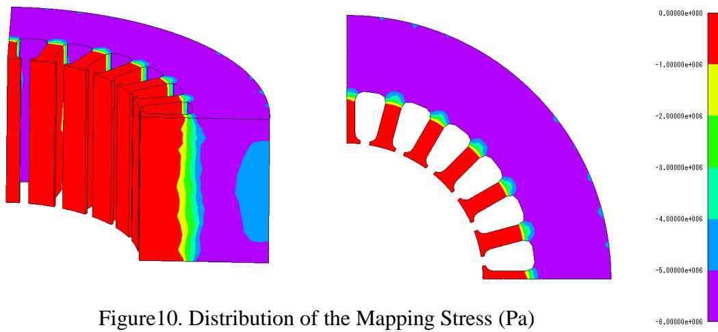
Figure10. Distribution of the Mapping Stress (Pa)
