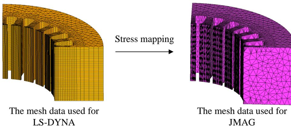
Figure6. FE Models used in each Analysis Step
