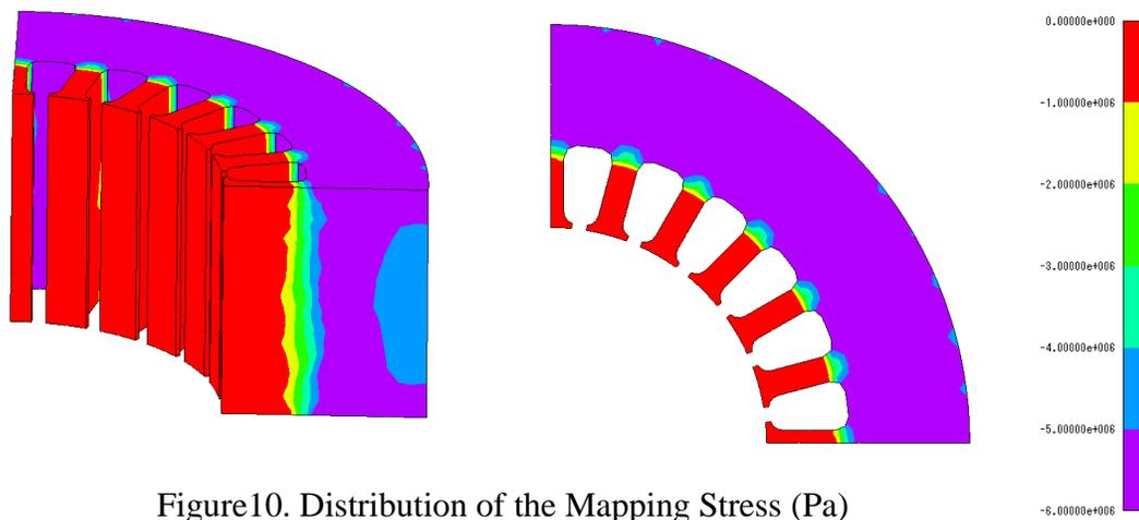
Figure10. Distribution of the Mapping Stress (Pa)
