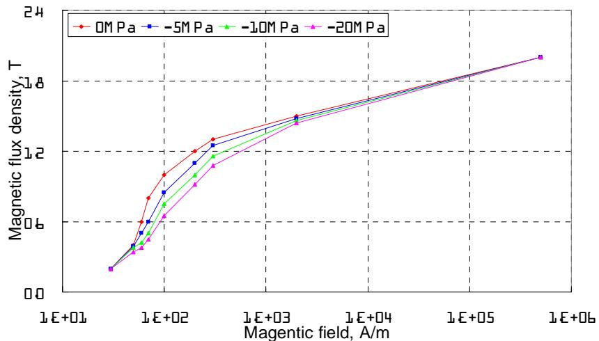
Figure3. Stress Dependent BH Curve (stator core)
