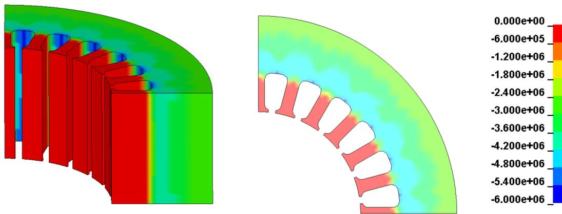
Figure8. Compressive Stress Distribution (Pa)
