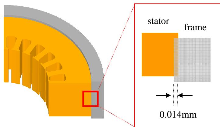
Figure5. Small Penetration between Stator core and Frame
