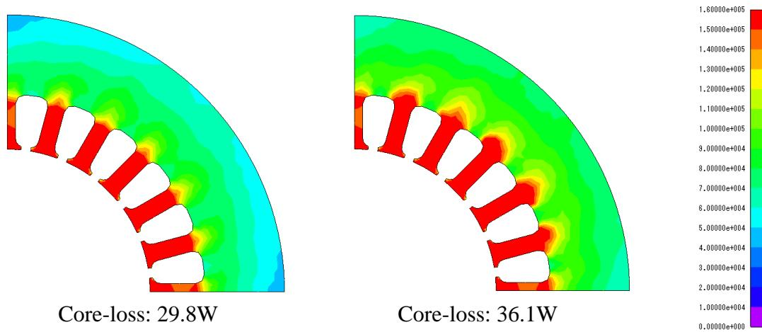
Figure 11. Iron Loss Density Distribution ( $\text{W}/\text{m}^3$ )
