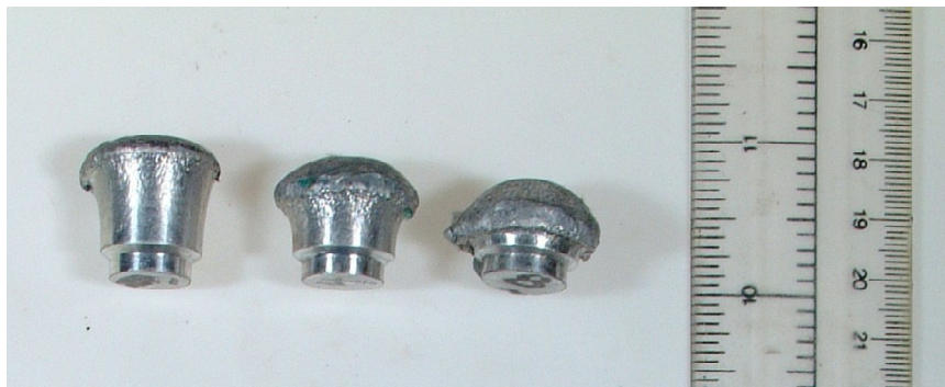
Figure 4 Deformed 6061-T6 aluminum projectiles after perforation 0.125, 0.25, and 0.5 inch thick (left-to-right) aluminum targets.
