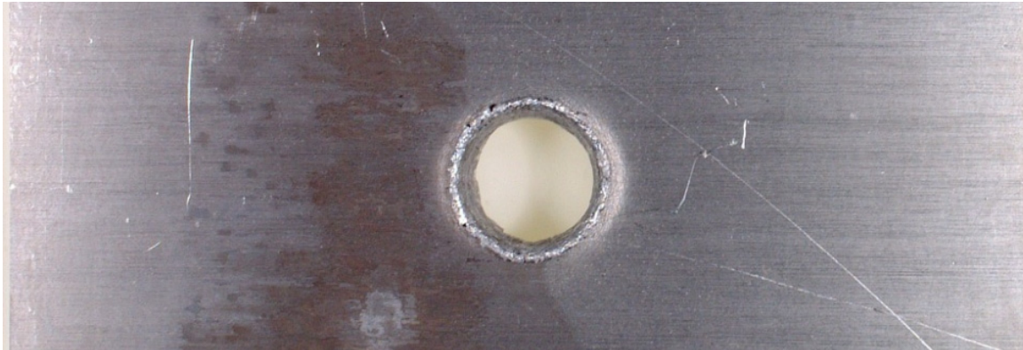
Figure 3 Side (upper image) and front (lower image) views of perforated 6061-T6 aluminum 0.5 inch thick target.
