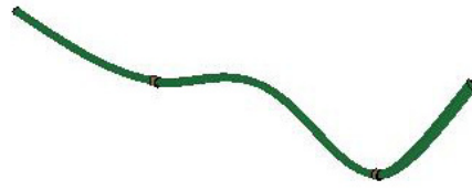
Figure 9 – Typical eigenmode shape for the improved fixture model
