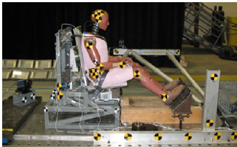
Figure 4: AORC Sled Test Set-up
