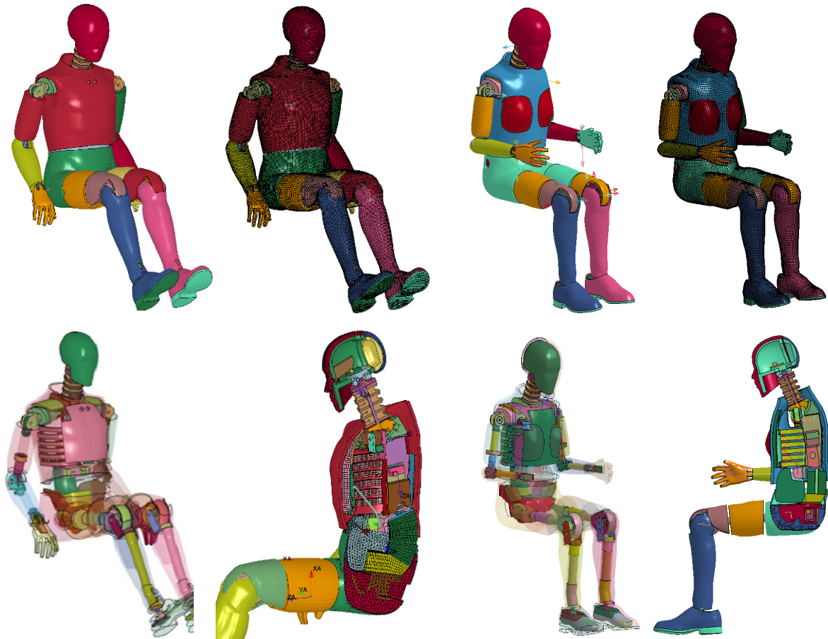
Hybrid III 50 th percentile FE model – 255000 elements Hybrid III 5 th percentile FE model – 200000 elements
