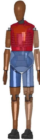
Figure 3: Hybrid III Rigid-FE 50 th male standing
