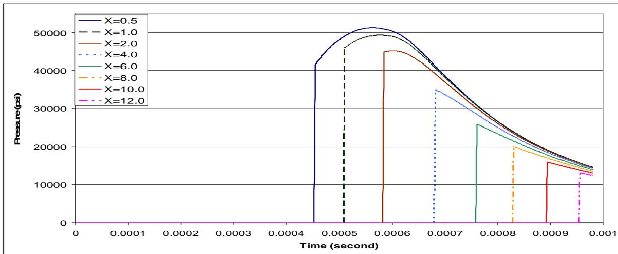
Figure 7 Plot of time-dependent pressure curves at selected locations (inch)
