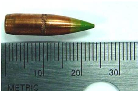
Figure 3 Display of M855 (5.56 mm) bullet
