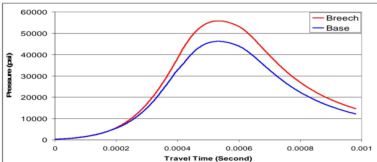
Figure 8 Computed breech and base pressure-time curves
