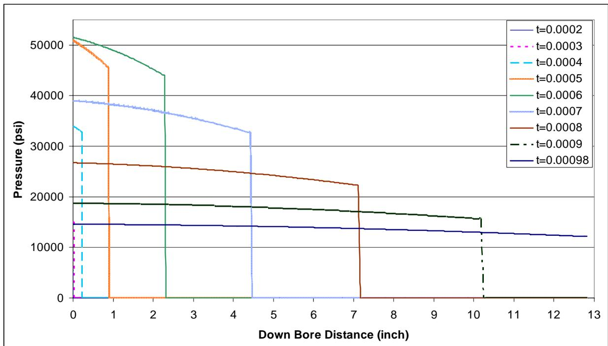
Figure 6 Plot of spatially varying pressure curves at selected time instant
