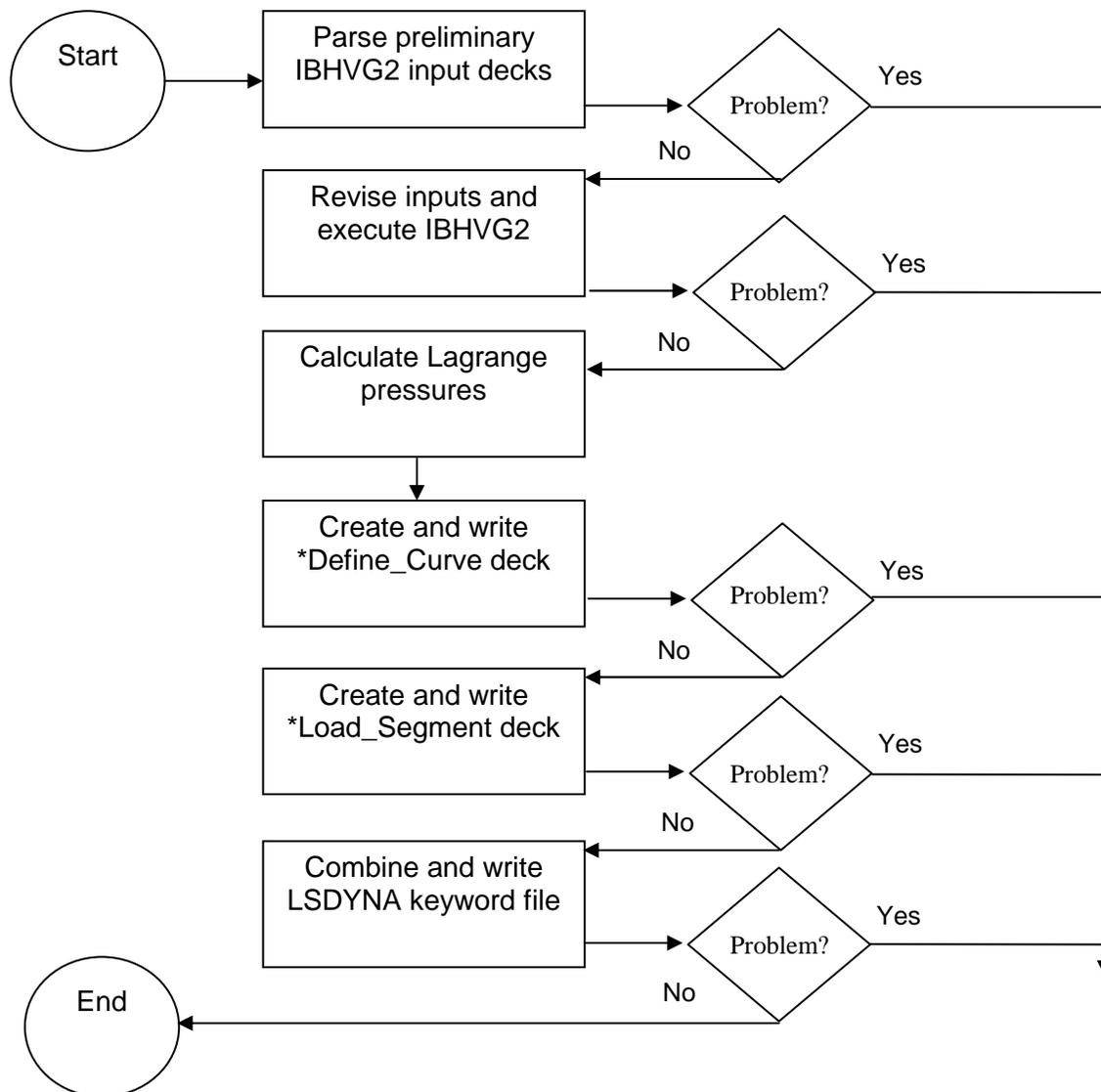
Figure 2 Flow chart of Pressurizer
