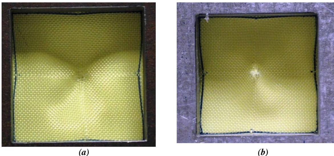
**Figure 4. Highest non-penetrating velocity sample for case 2 (a) front view (b) rear view**
