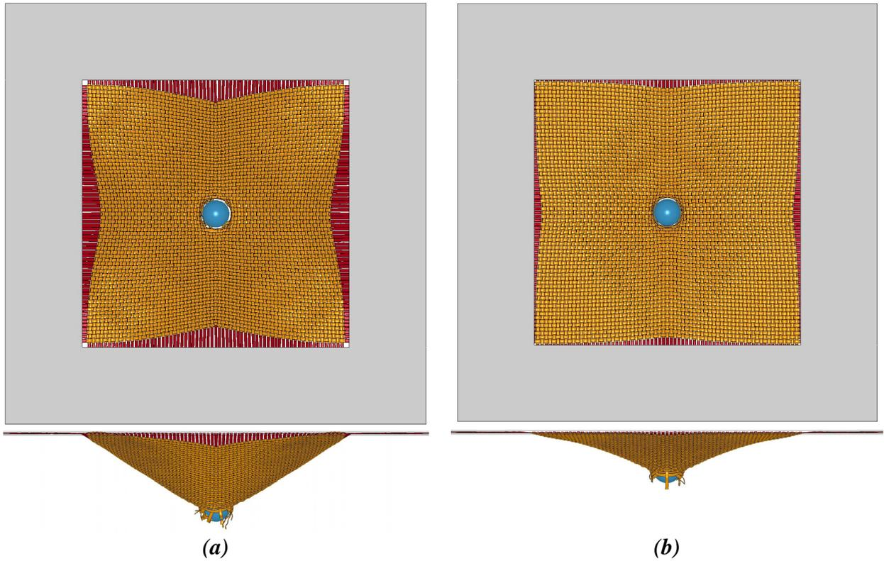
Figure 9. Sample deformation state for case with yield stress of (a) 20 MPa (b) 200 MPa
