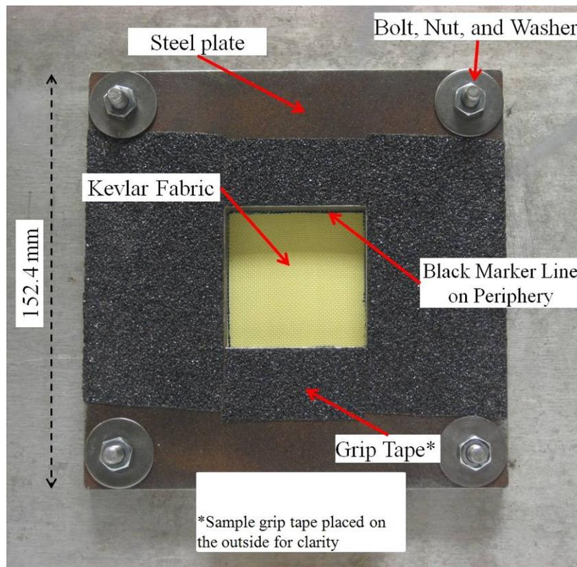
Figure 1. Experimental test setup
