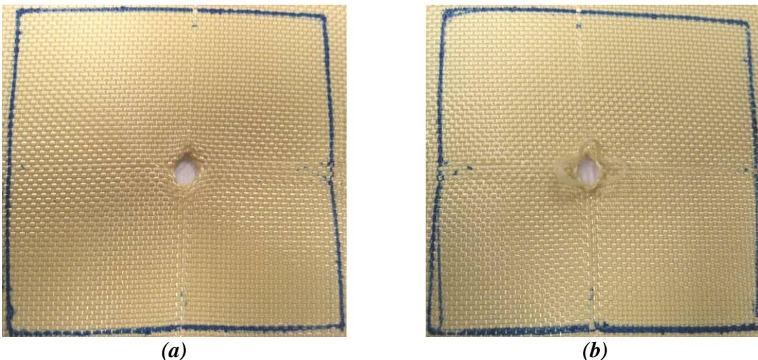
**Figure 5. Lowest completely penetrating velocity sample for case 1**
