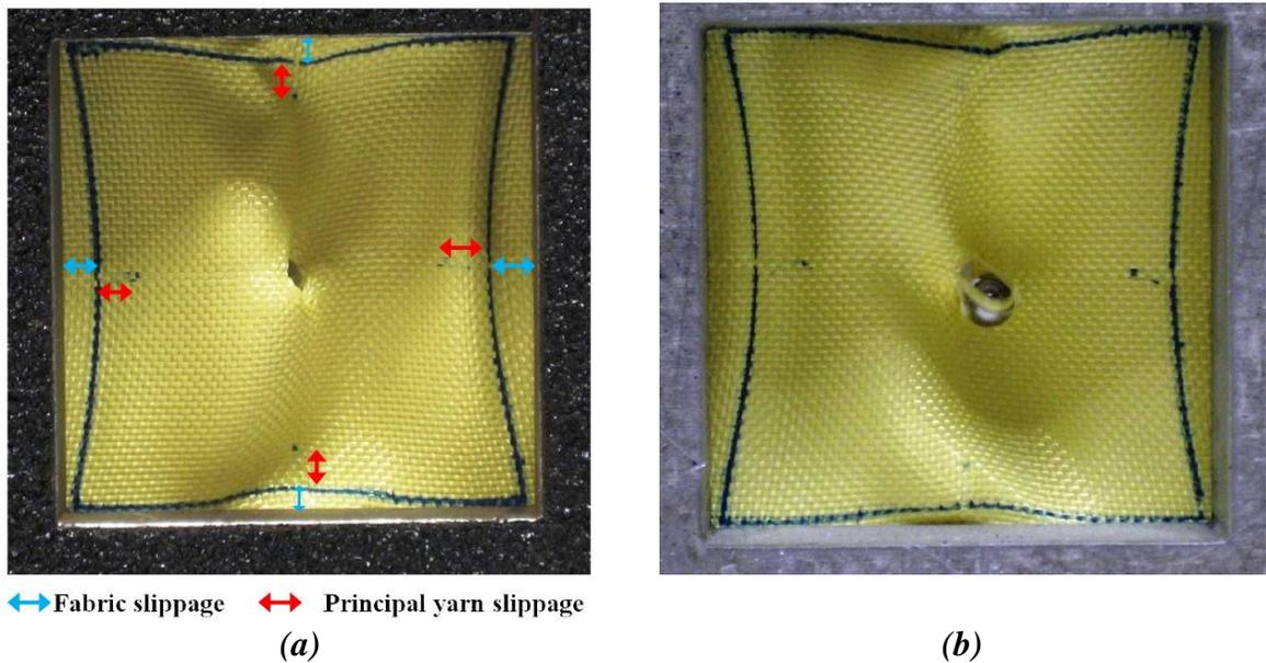
**Figure 3. Highest non-penetrating velocity sample for case 5 (a) front view (b) rear view**
