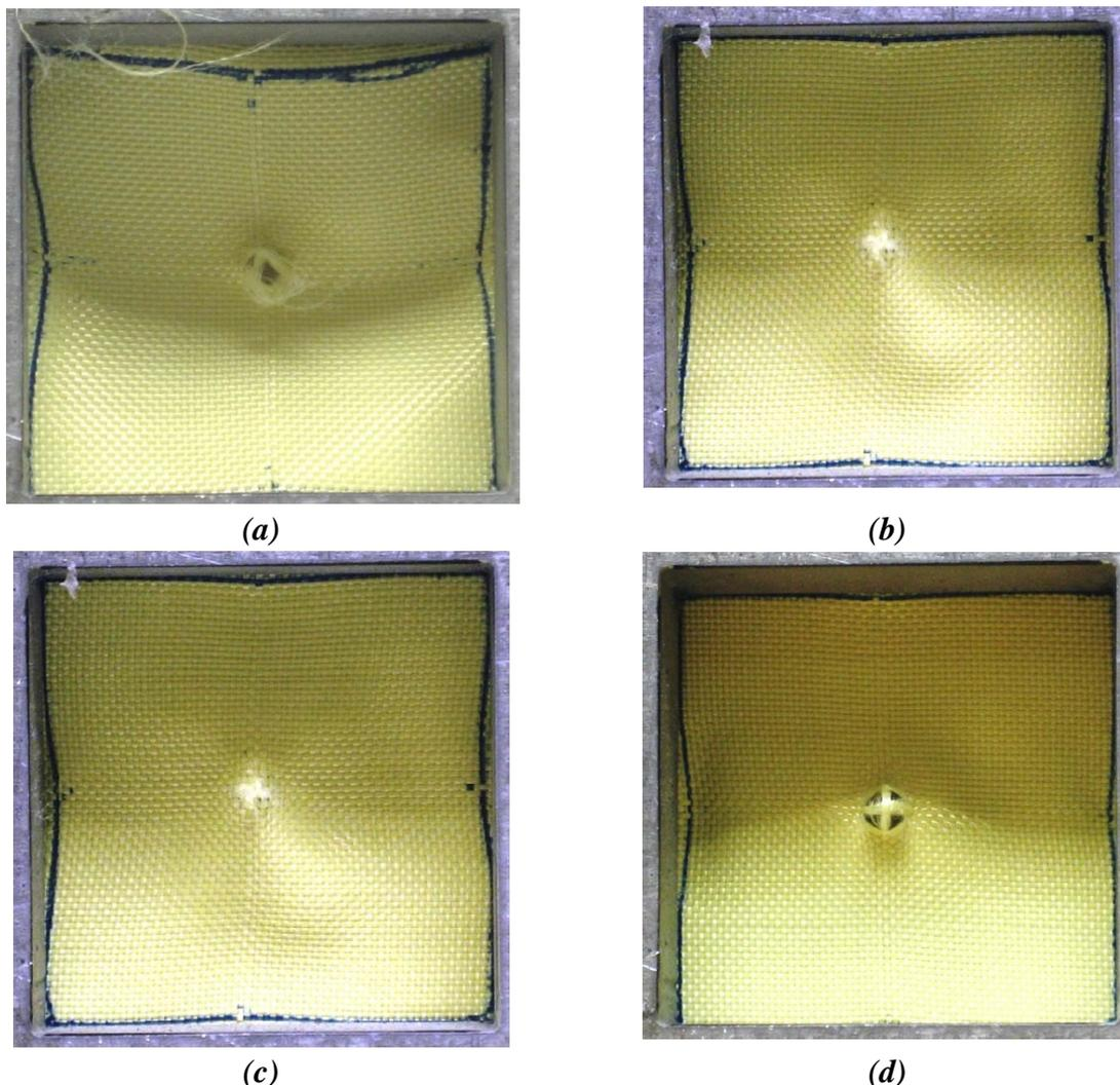
**Figure 2. Rear view of the highest non-penetrating velocity samples for
