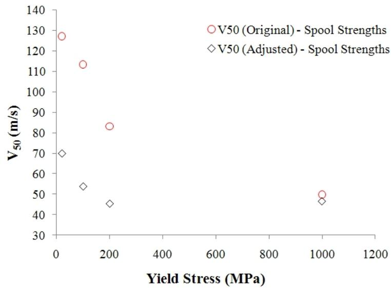
Figure 10.  $V_{50}$  velocities as a function of yield stress
