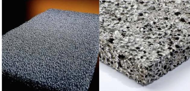
Fig. 1: foam panels – M-PORE and ALPORAS [7]
