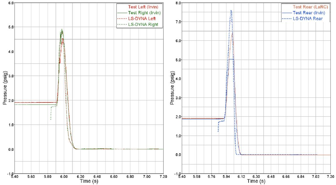
**Figure 14: Vertical Velocity Drop Test- Test Data and LS-DYNA Model Prediction- Airbag Pressure Time History**
