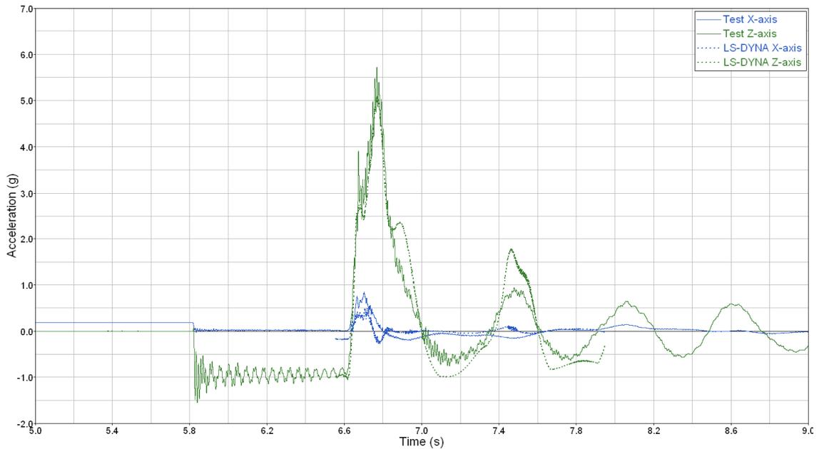
**Figure 15: Vertical Velocity, 10 Degree Pitch Drop Test- Test Data and LS-DYNA Model Prediction- Acceleration Time History**
