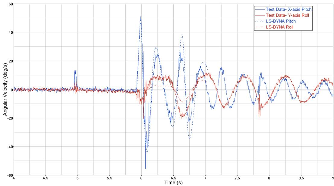
**Figure 13: Vertical Velocity Drop Test- Test Data and LS-DYNA Model Prediction- Angular Velocity Time History**
