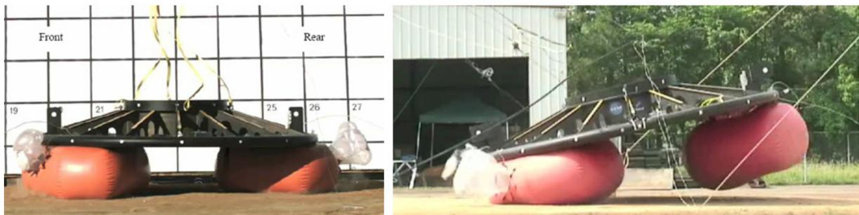
**Figure 11: Gen1 Drop Testing Images**
