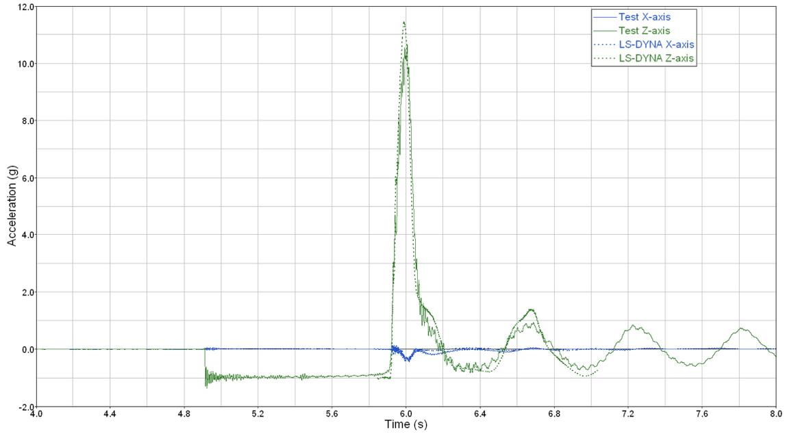
**Figure 12: Vertical Velocity Drop Test- Test Data and LS-DYNA Model Prediction- Acceleration Time History**
