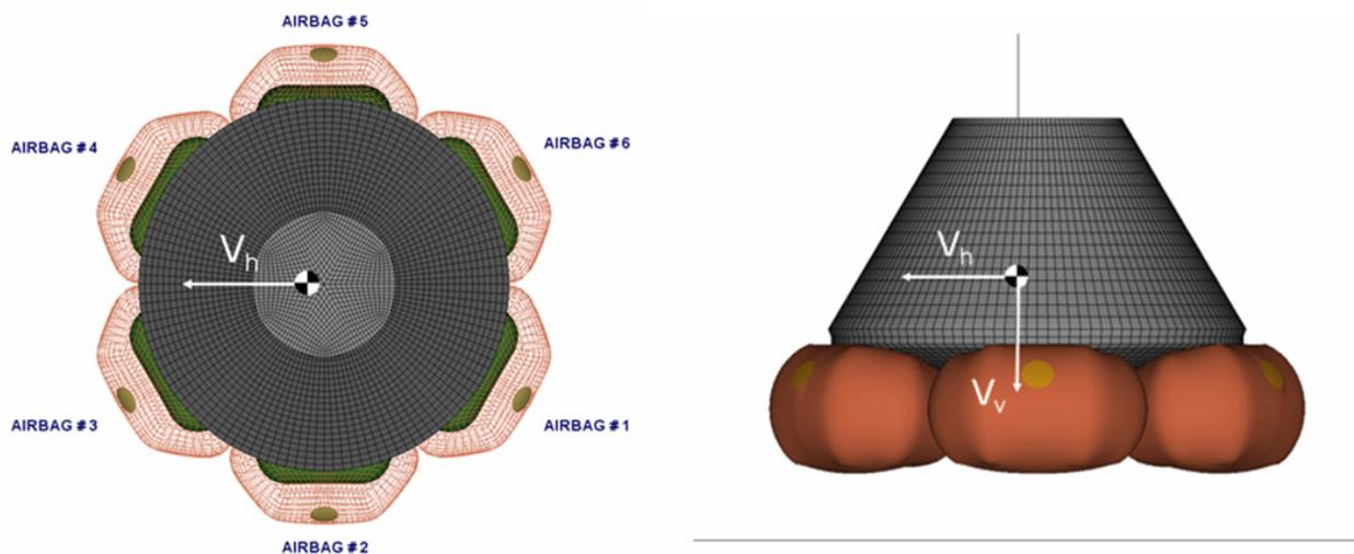
**Figure 4: Airbag System and Landing Velocity Definitions**
