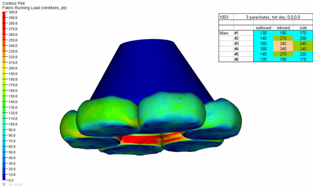
**Figure 7: Gen2 Fabric Stress Contours**
