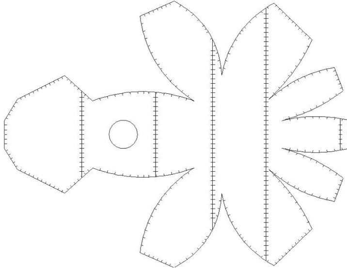
**Figure 8: Gen2 Main Airbag Flat Pattern**
