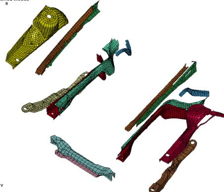
Fig. 3: Thickness design variables (with exploded view).
