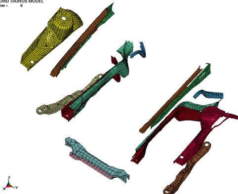
Fig. 3: Thickness design variables (with exploded view).
