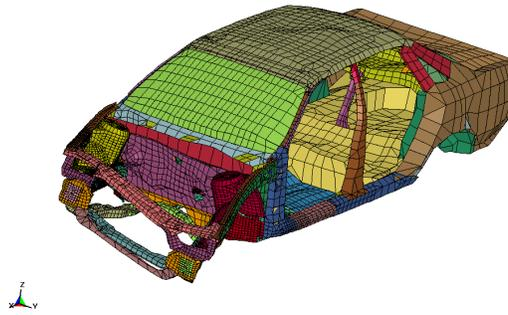
Fig. 1: Finite element crash model.
