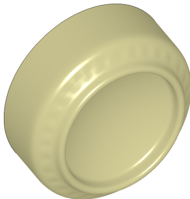
Figure 3. Typical beverage can dome showing profile wrinkles.
