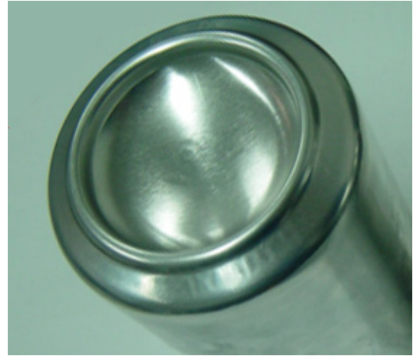
Figure 2. Photograph of beverage can showing dome profile wrinkles.
