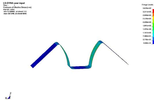
Springback using Inertia Relief
