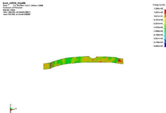
For binder wrap applications we use the new `*CONTROL_IMPLICIT_FORMING` keyword with a “2” in the first field. The difference between “1” and “2” is that for applications we expect to take only one time step we use “1”, otherwise we recommend “2”.
