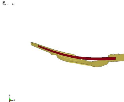
To make constructing LS-DYNA keyword input files easier we have added a new implicit keyword `*CONTROL_IMPLICIT_FORMING`. Using the value of 1 in the first field for this keyword, with no other implicit keywords, allows gravity loading problems to converge in one time step and few nonlinear iterations.
