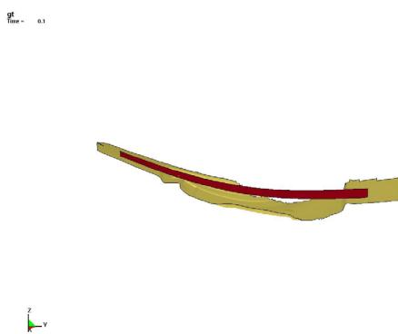
To make constructing LS-DYNA keyword input files easier we have added a new implicit keyword \*CONTROL\_IMPLIPLICIT\_FORMING. Using the value of 1 in the first field for this keyword, with no other implicit keywords, allows gravity loading problems to converge in one time step and few nonlinear iterations.
