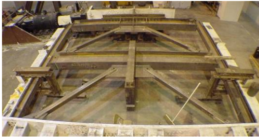
a) Test setup for SCBF
