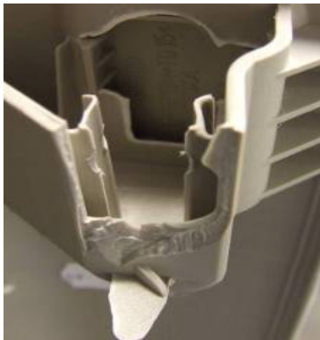
Figure 3 Common failure mode – local trim break
