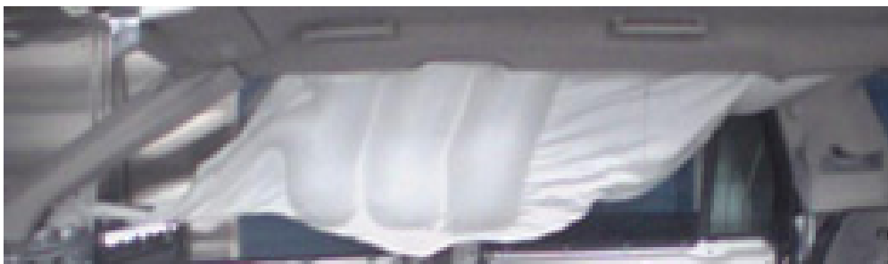
Figure 1 Common failure mode – curtain airbag hang-up
