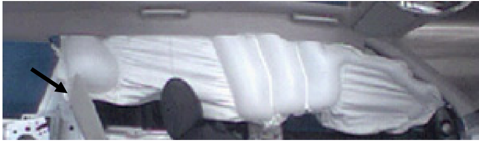
Figure 2 Common failure mode – C-pillar trim detachment
