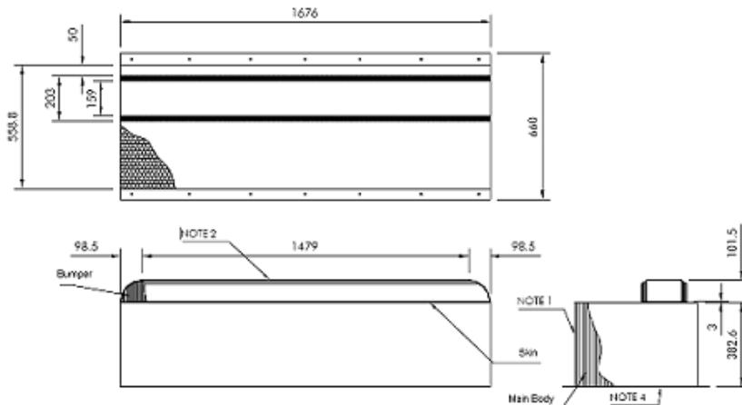
Figure 1. NHTSA Barrier Parts and General Dimensions
