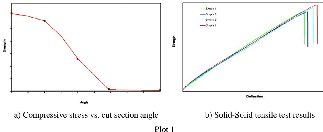
a) Compressive stress vs. cut section angle
