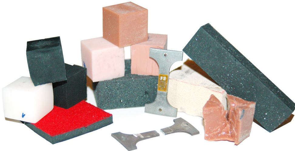
Figure 1: Material test samples of the WorldSID.
