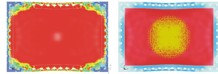
Figure 17. Composite impact case 147.5m/s – matrix cracks and fibre failure (left)
