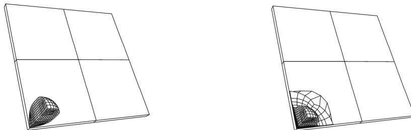
Figure 3a. Rigid wall bird strike impact, 250m/s, 1kg (time = 0μsec)
