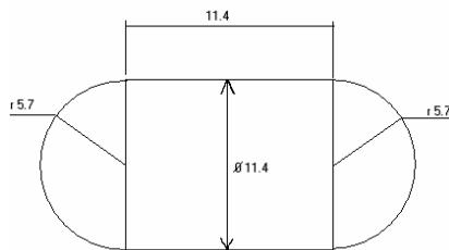
Figure 1: Bird Model Geometry (all dimensions are in cm) [1]
