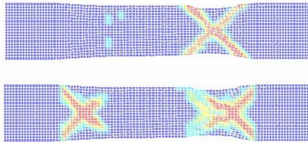
Figure 10. Coupon simulation for tensile-shear specimen (shear failure, top)
