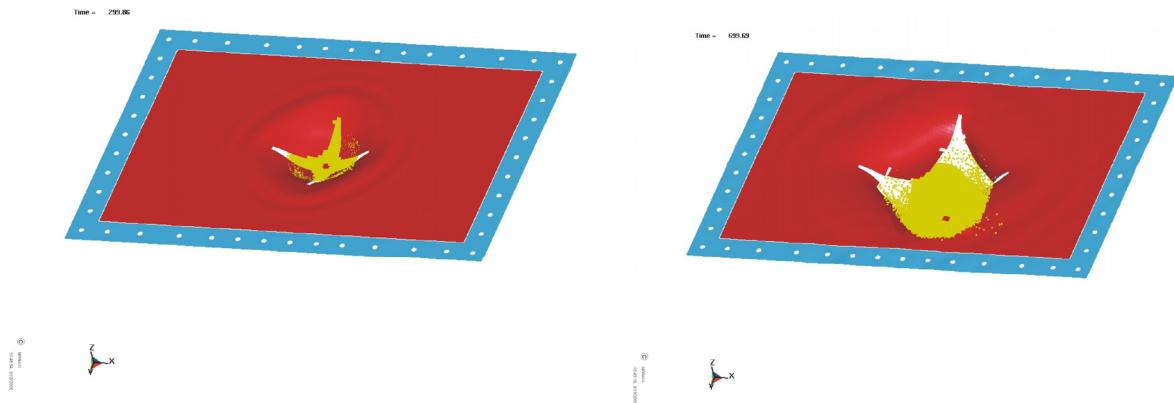
Figure 19. Composite impact case 245m/s – deformed shape time 300μsec (left)
