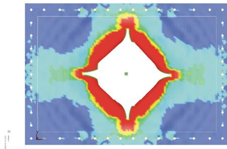
Figure 23. Composite impact case 245m/s – matrix and fibre damage
