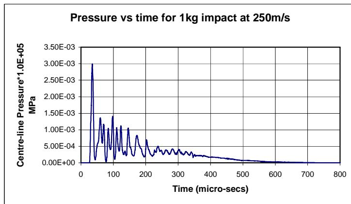
Figure 4. Pressure ( $\times 10^5$ MPa) vs. time (μsec) history for centre-line element of bird 250m/s: coarse Lagrangian bird mesh (704 solid finite elements)
