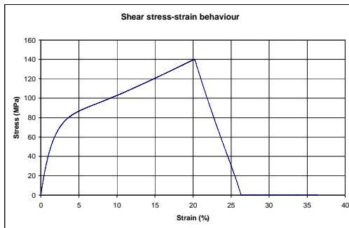
Figure 7. Shear stress-strain behaviour for woven glass
