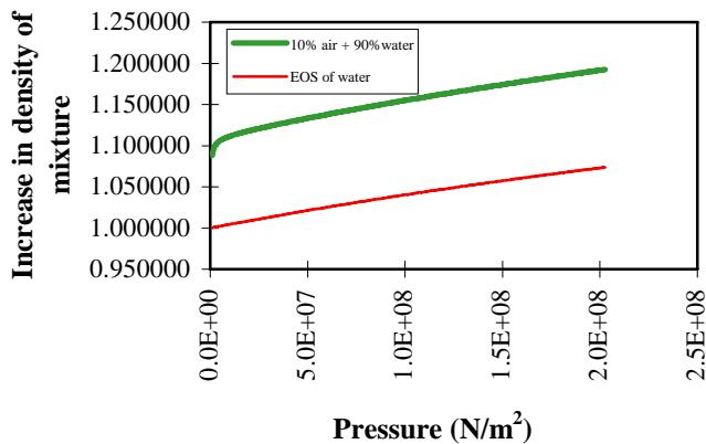
Figure 2: Equation of State for bird material in relation to the EOS of water [1]
