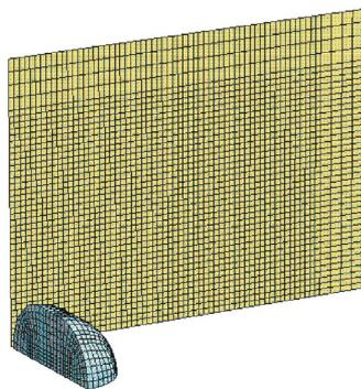
Figure 12. Composite panel FE shell mesh
