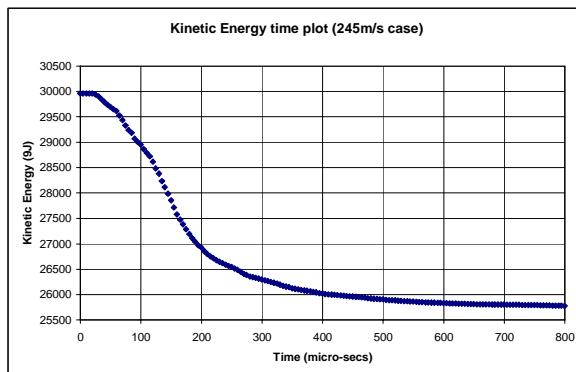
Figure 22. Kinetic Energy for composite bird impact case at 245m/s using SPH
