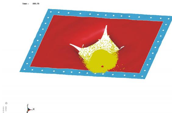
Figure 21. Impact case 245m/s – deformed shape time 900μsec
