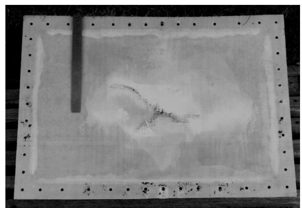
Figure 16. Impact case 245m/s – experimental deformed shape (right)
