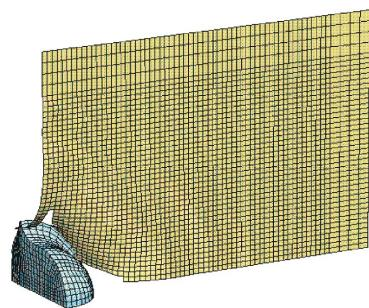
Figure 13. Impact case 147.5m/s – deformed shape (left)
