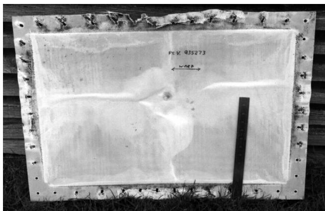
Figure 15. Impact case 147.5m/s – experimental deformed shape (left)
