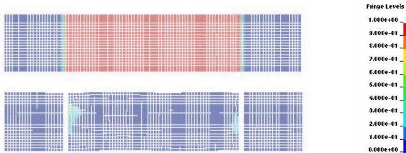
Figure 8. Coupon simulation for tensile specimen (matrix cracks, top)
