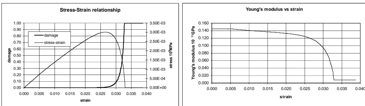
Figure 5. Direct stress-strain relationship for woven glass model (left)
