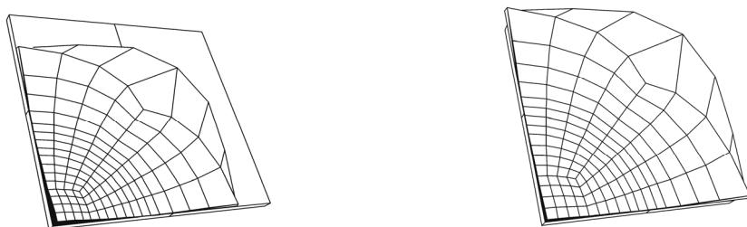
Figure 3c. Rigid wall bird strike impact, 250m/s, 1kg (time = 600μsec)
