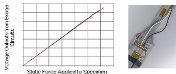
Figure 4. Quasi-static calibration curves
