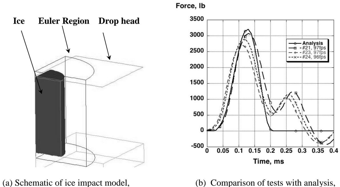
Figure 13. LS-DYNA ice model and simulation results compared with test data.
