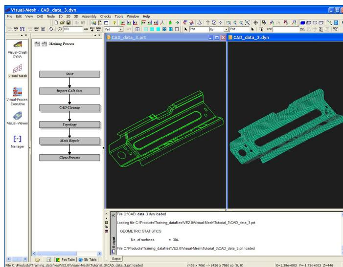
It automatically cleans up the CAD data to get a good topology from CAD and in turn a good quality mesh. The template can be executed either in **Auto mode** or **Interactive mode**. In **Auto mode** it will be executed with default values and no user interaction is needed.
