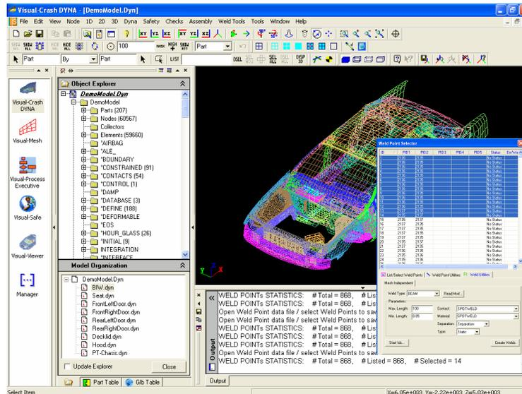
One of the most valuable features is the weld comparison tool to compare master weld file and/or mesh independent welds between two different models. The feature identifies and displays the difference between two different models. The user can view the matching and/or un-matching welds, delete or copy the welds from one model to another.
