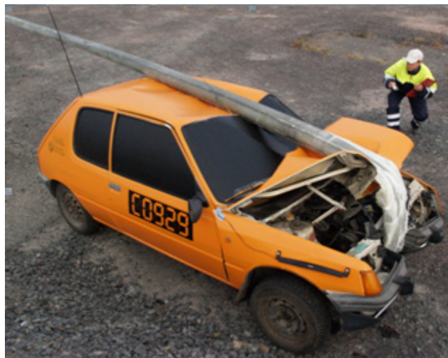
Fig. 2. Deformed column and vehicle after impact of 100 km/h. Impact tests performed by Helsinki University of Technology, Laboratory of Highway Engineering
