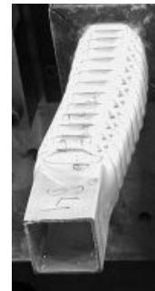
Figure 1. Profile D1-10, L = 1201 mm, v_0 = 13 m/s, t = 3.5 mm: (a) force versus deformation, (b) deformed geometry (Jensen [2]).
