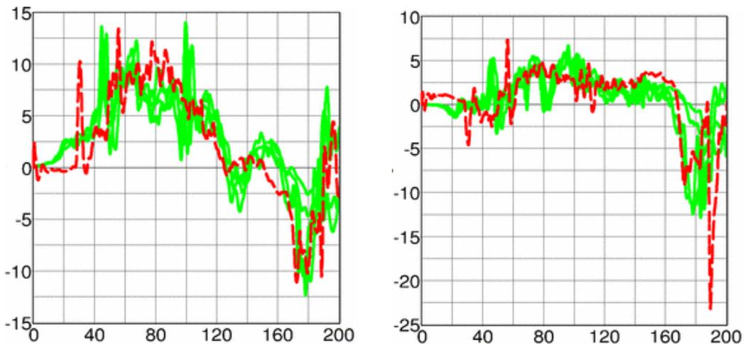
Figure 19: Spine acceleration [g] vs. time [ms] at T8. Left: x-acceleration. Right: z-acceleration.
