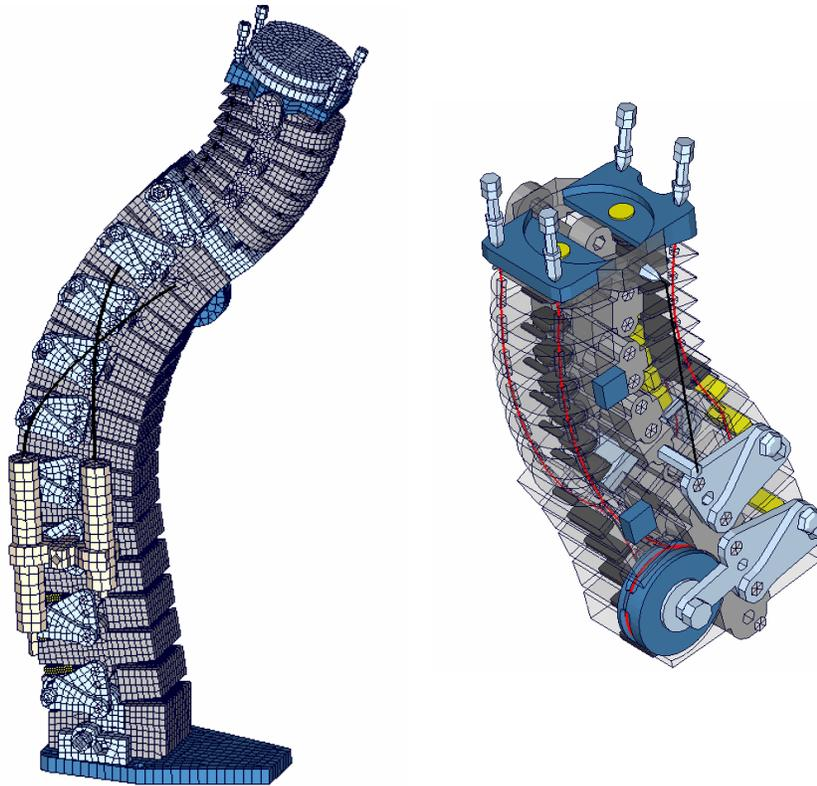
Figure 6: Selected parts of dummy model. Left: Spine and neck model. Right: Neck model, with steel cable in red.
