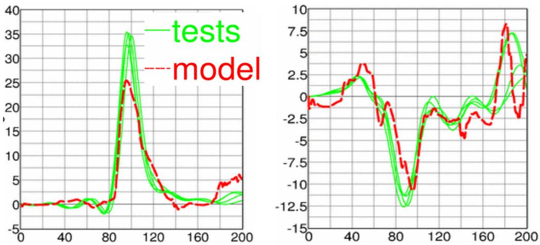
Figure 16: Head acceleration [g] vs. time [ms]. Left: x-acceleration. Right: z-acceleration.
