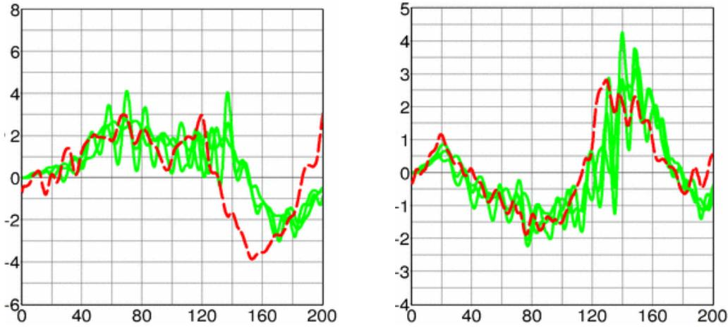
Figure 10: Upper spine acceleration [g] vs. time [ms] at T1. Left: x-acceleration. Right: z-acceleration.
