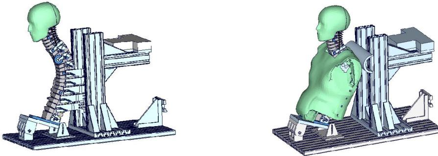
Figure 3: Left: BioRID II component test with supported spine. Right: Component test of assembled thorax.
