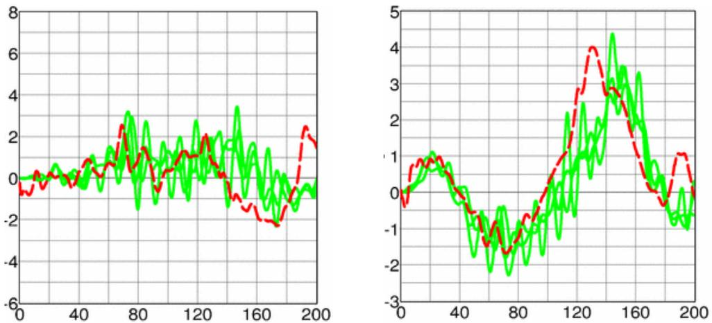
Figure 9: Neck acceleration [g] vs. time [ms] at C4. Left: x-acceleration. Right: z-acceleration.
