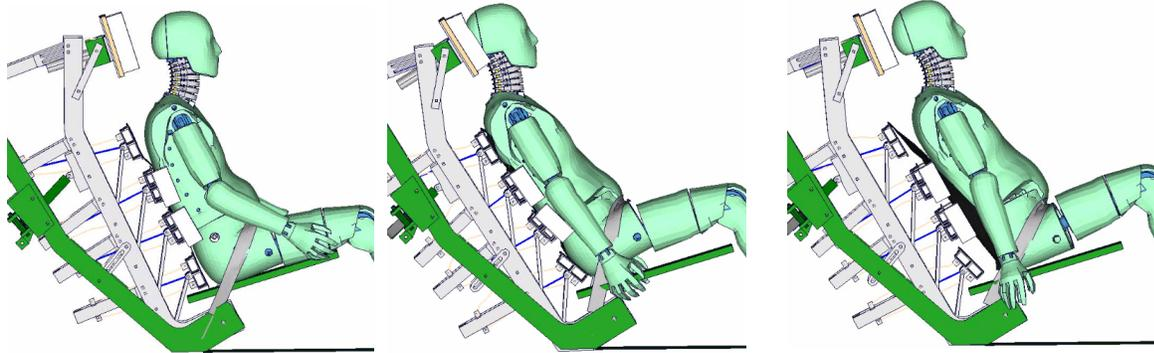
Figure 15: Behavior of dummy model in simplified seat test.
