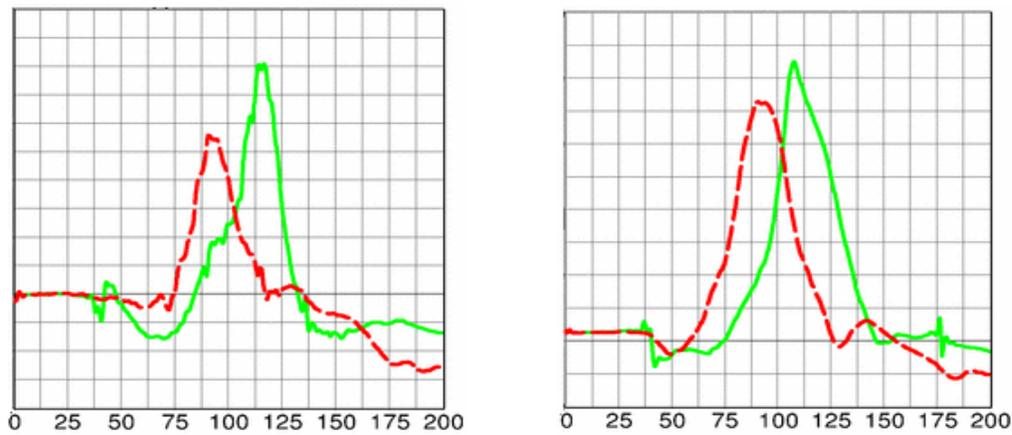
Figure 28: Upper and lower neck x-force vs. time [ms]. Influence of back rest stiffness.
