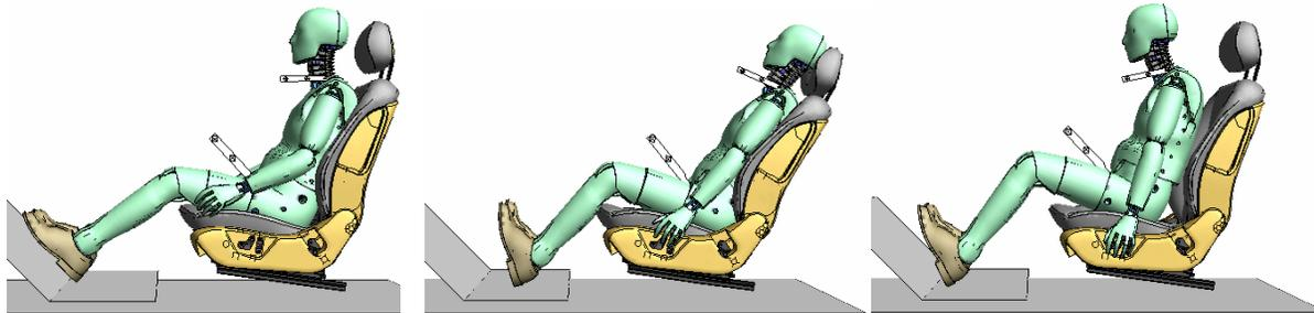
Figure 25: Dummy in seat model at time: 0, 105, and 200 ms.
