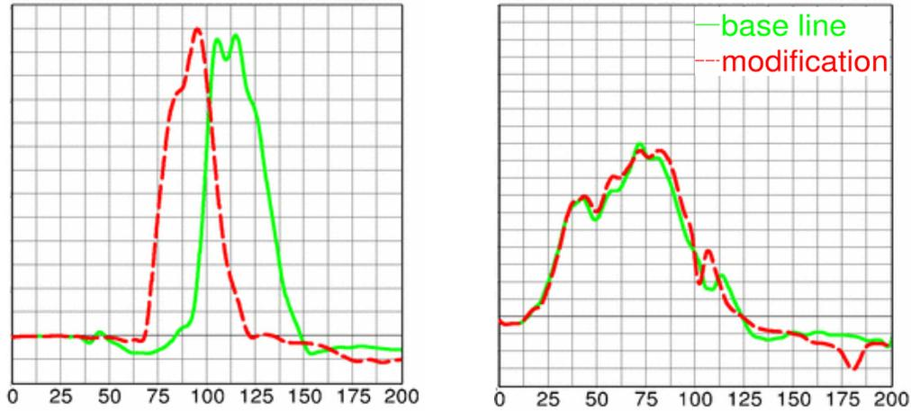
Figure 27: Head and pelvis x-acceleration vs. time [ms]. Influence of back rest stiffness.
