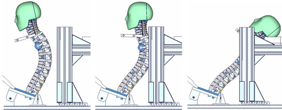
Figure 7: Spine, neck, and head during component test at 0, 90, and 200 ms.
