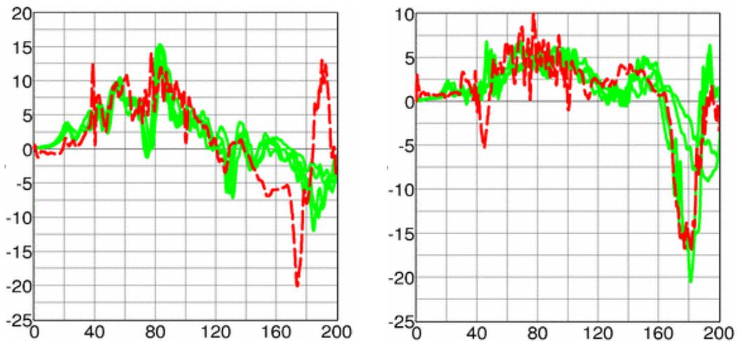
Figure 20: Spine acceleration [g] vs. time [ms] at L1. Left: x-acceleration. Right: z-acceleration
