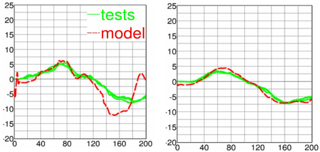
Figure 14: Left: Upper neck moment [Nm] along y vs. time [ms]. Right: Lower neck moment [Nm] along y vs. time [ms].
