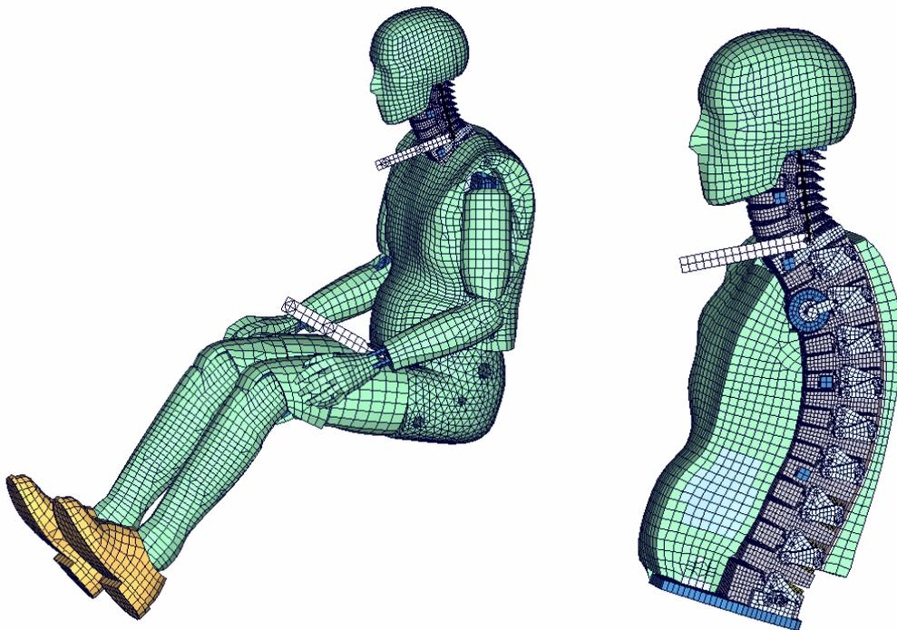
Figure 5: FAT LS-DYNA BioRID II dummy model. Left: completely assembled model. Right: Thorax and head model cutted along the spine.
