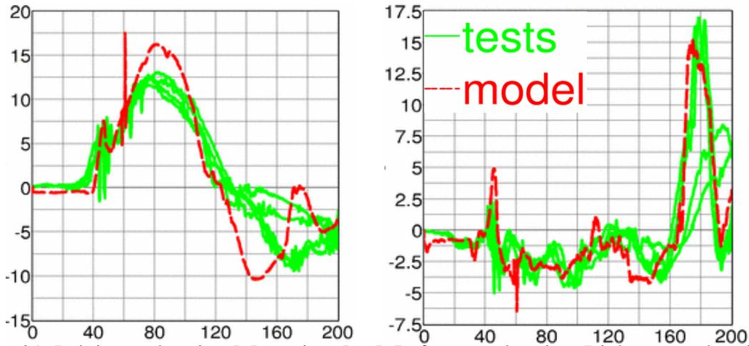
Figure 21: Pelvis acceleration [g] vs. time [ms]. Left: x-acceleration. Right: z-acceleration
