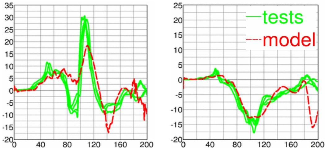
Figure 24: Left: Upper neck moment [Nm] along y axis vs. time [ms]. Right: Lower neck moment [Nm] along y axis vs. time [ms].
