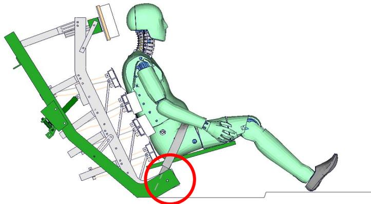
Figure 4: Simplified seat model to perform the assembled dummy tests.
