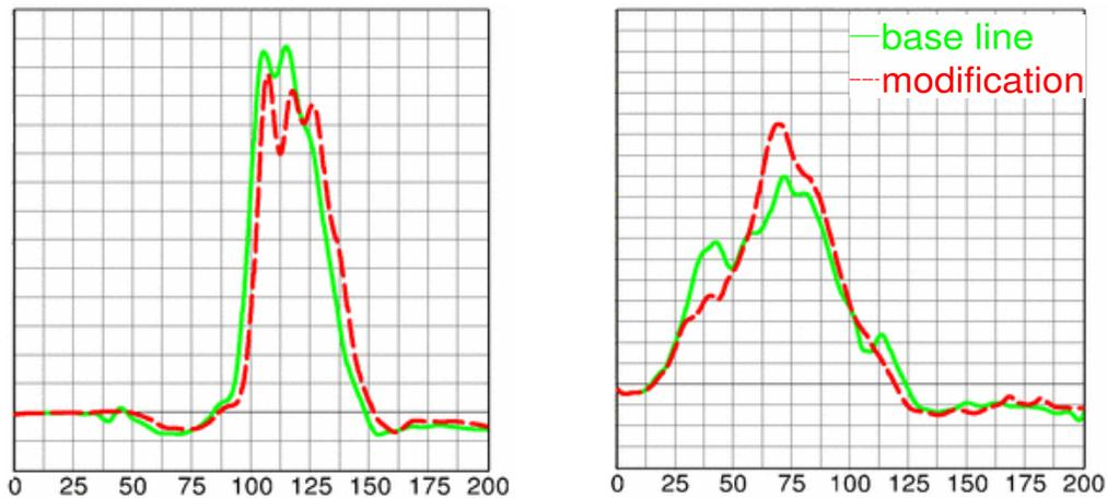
Figure 30: Head and pelvis x-acceleration vs. time [ms]. Influence of friction.
