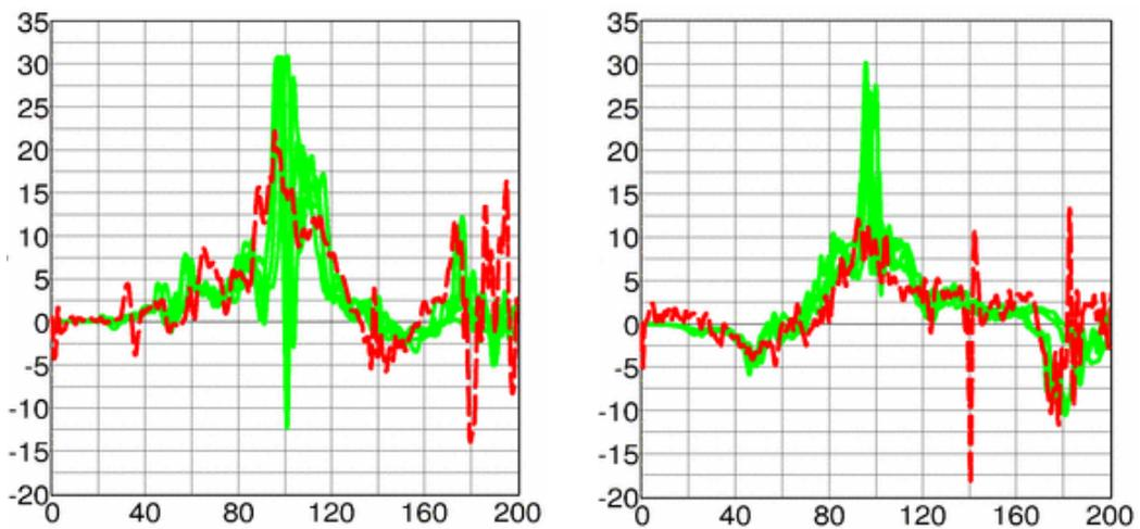
Figure 17: Neck acceleration [g] vs. time [ms] at C4. Left: x-acceleration. Right: z-acceleration.
