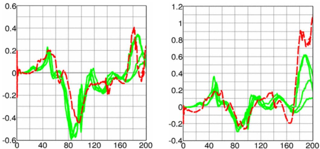
Figure 23: Lower neck force [kN] vs. time [ms]. Left: Force in x. Right: Force in z.
