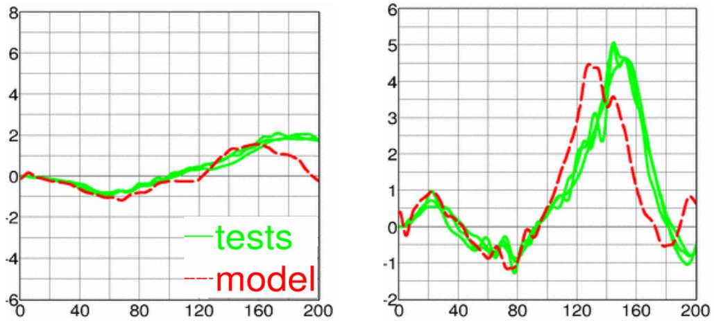
Figure 8: Head acceleration [g] vs. time [ms]. Left: x-acceleration. Right: z-acceleration.
