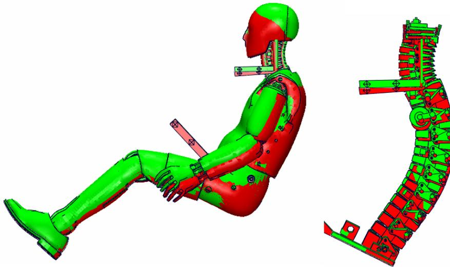
Figure 26: Varying initial position due to different types of pre-simulations (Green: Base line. Red: Complete deformable positioning). Left: Complete model. Right: Spine and neck model.
