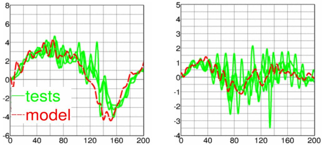
Figure 11: Spine acceleration [g] vs. time [ms] at T8. Left: x-acceleration. Right: z-acceleration.
