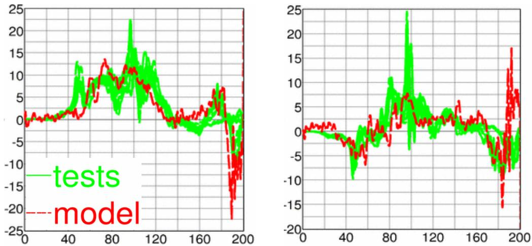
Figure 18: Upper spine acceleration [g] vs. time [ms] at T1. Left: x-acceleration. Right: z-acceleration.
