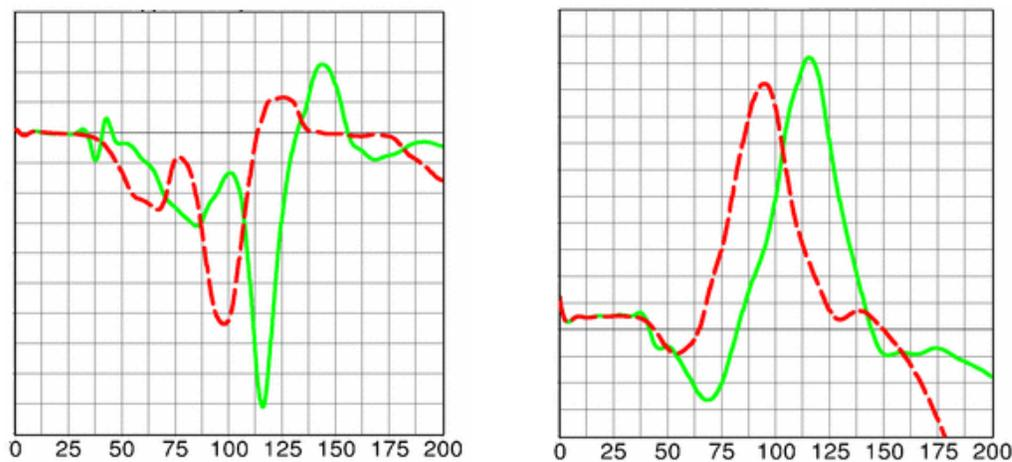
Figure 29: Upper and lower neck y-moment vs. time [ms]. Influence of back rest stiffness.
