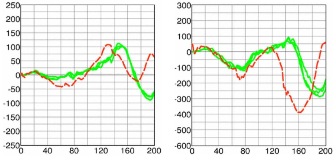
Figure 13: Lower neck force [N] vs. time [ms]. Left: Force in x. Right: Force in z.
