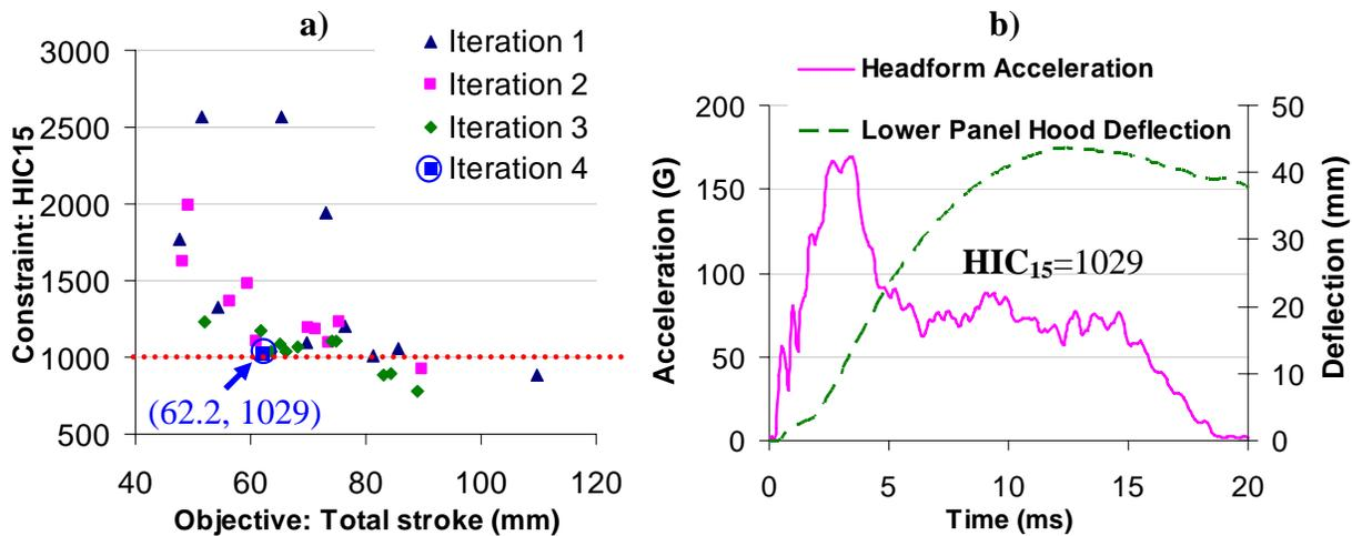
**Figure 8.** a) Trade-off of HIC<sub>15</sub> versus Total stroke b) The time histories of headform acceleration and the deflection of Hood Lower Panel in last simulation (the fourth iteration)
