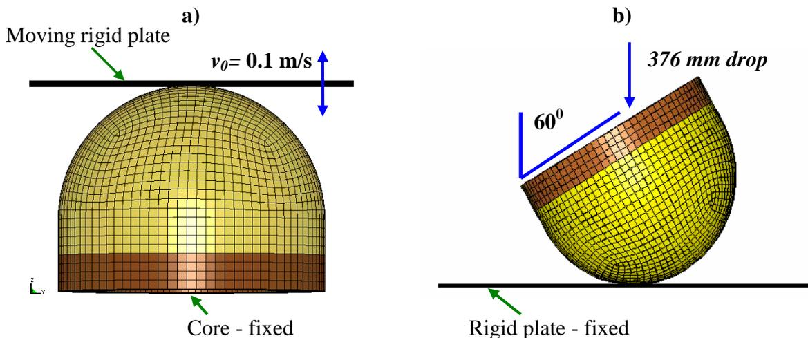
**Figure 2.** Test set-ups of skin validation tests; a) quasi-static test; b) dynamic test
