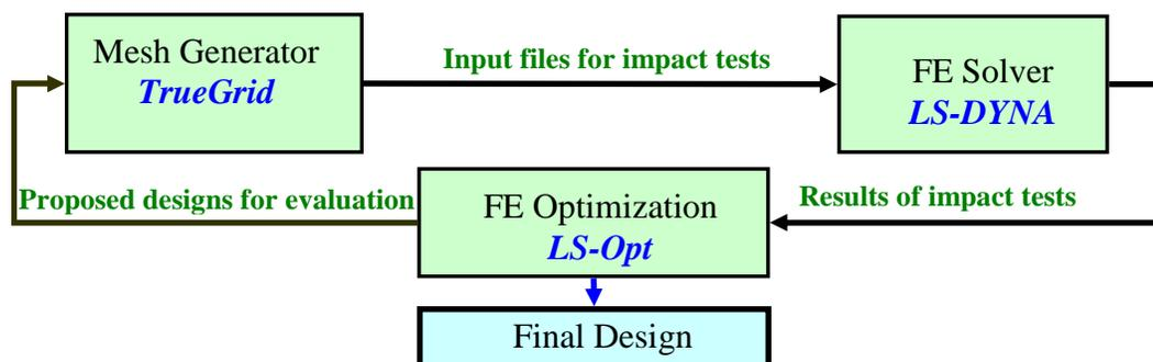
Figure 5. Schematic automatic geometry optimization of hood design
