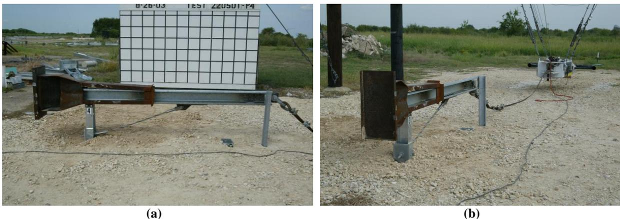
FIGURE 6 Pendulum test setup for applying loads on the cable anchor.
