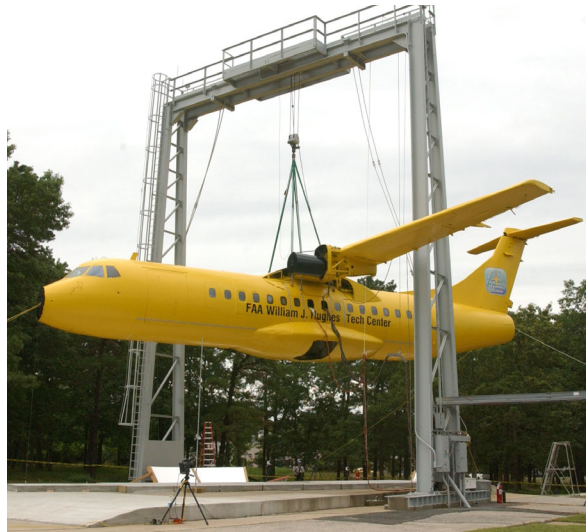
Figure 1. Pre-test photograph of the ATR42 aircraft, raised to a drop height of 14 feet.
