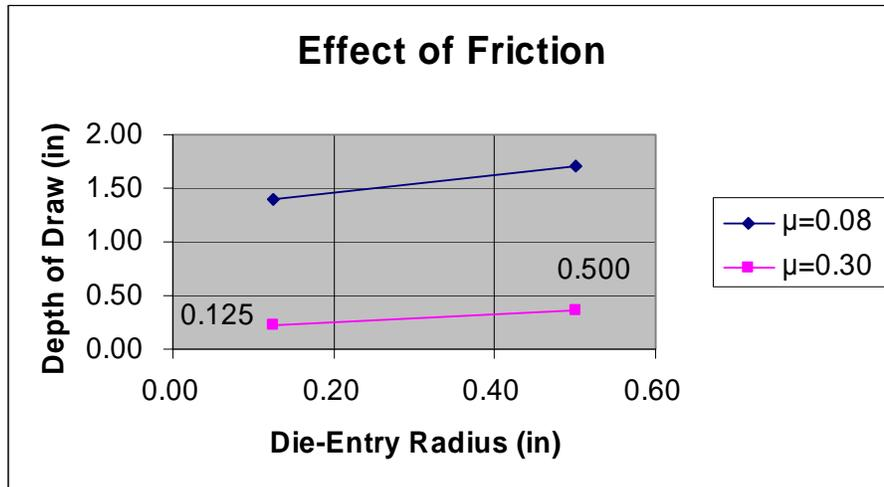
**Figure 7** Influence and interaction of friction and die-entry radius
