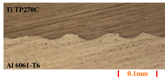
Figure 6. One side of the line welding of Ti TP270C to Al 6061-T6
