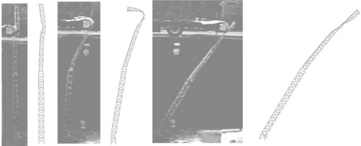
Fig. 3: Impact events from FEA simulation and full-scale test. Direction: Side, Top mass: 5.44 kg, Velocity: 140 km/h (Case Study 1)
