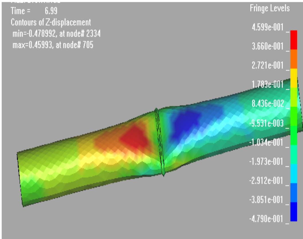
Figure 9. Loss of stability of the tube under shrinkage forces
