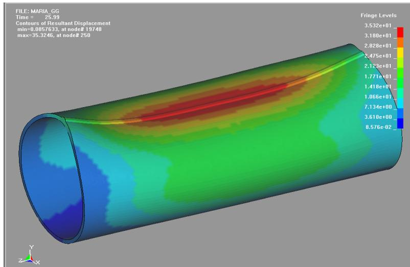
Figure 8. Welded tube structure under shrinkage forces applied to the longitudinal weld
