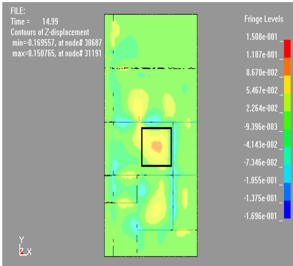
Figure 12. The area of maximum z-displacement found by means of application of shrinkage forces to the new and old welds
