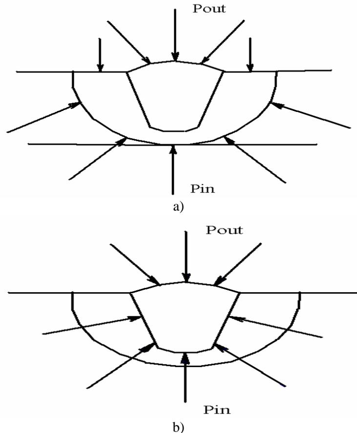
Figure 1. Scheme of the transversal loads applied to the plastic zone near weld ( $P_{in}$ ,  $P_{out}$  are an internal and an external forces)
