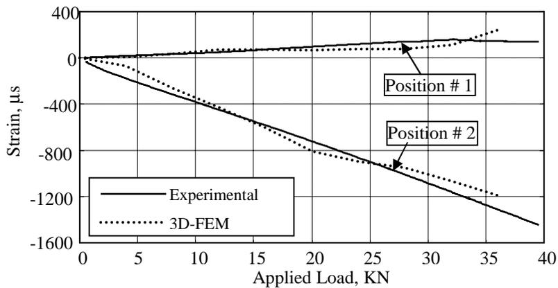
b. Measured and Calculated Strains.
