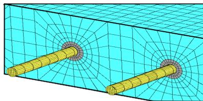
b. Detailed Mesh of Dowels and Surrounding Concrete.
