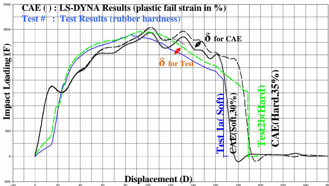
Figure 9. F-D: Test Vs. CAE and Hard (H) Vs. Soft(S) Rubber Mount
