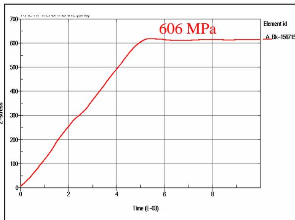
Figure 5. Z-Stress of Element “s”
