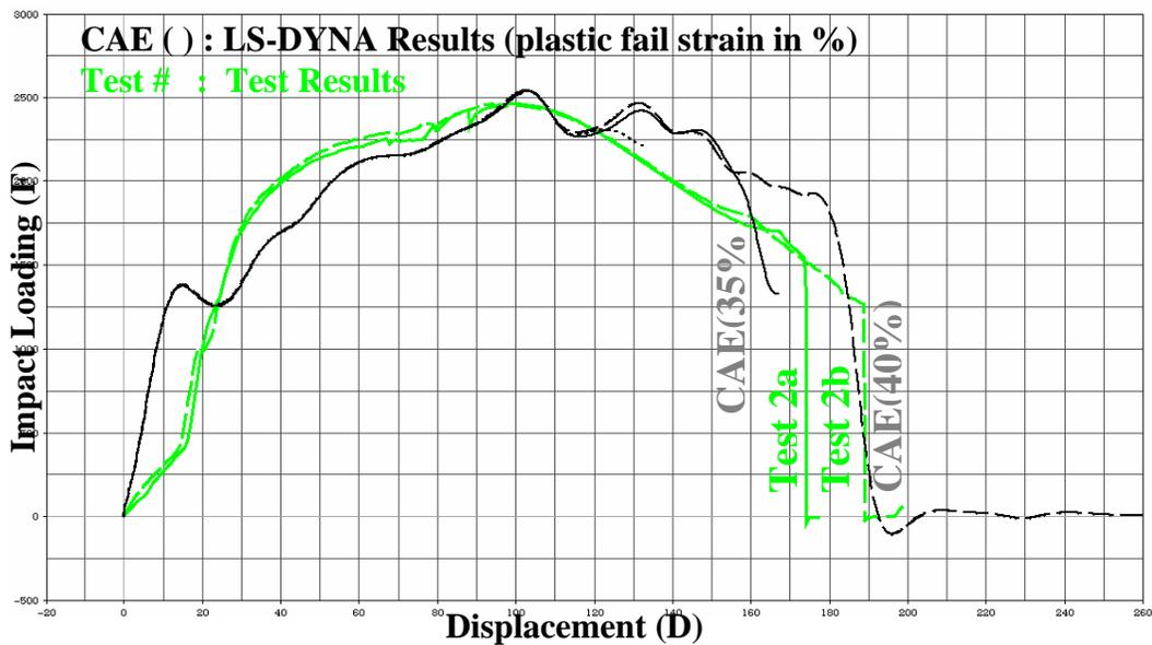
Figure 8. F-D Curves for Test and CAE analysis for Hard (H) Rubber Mount
