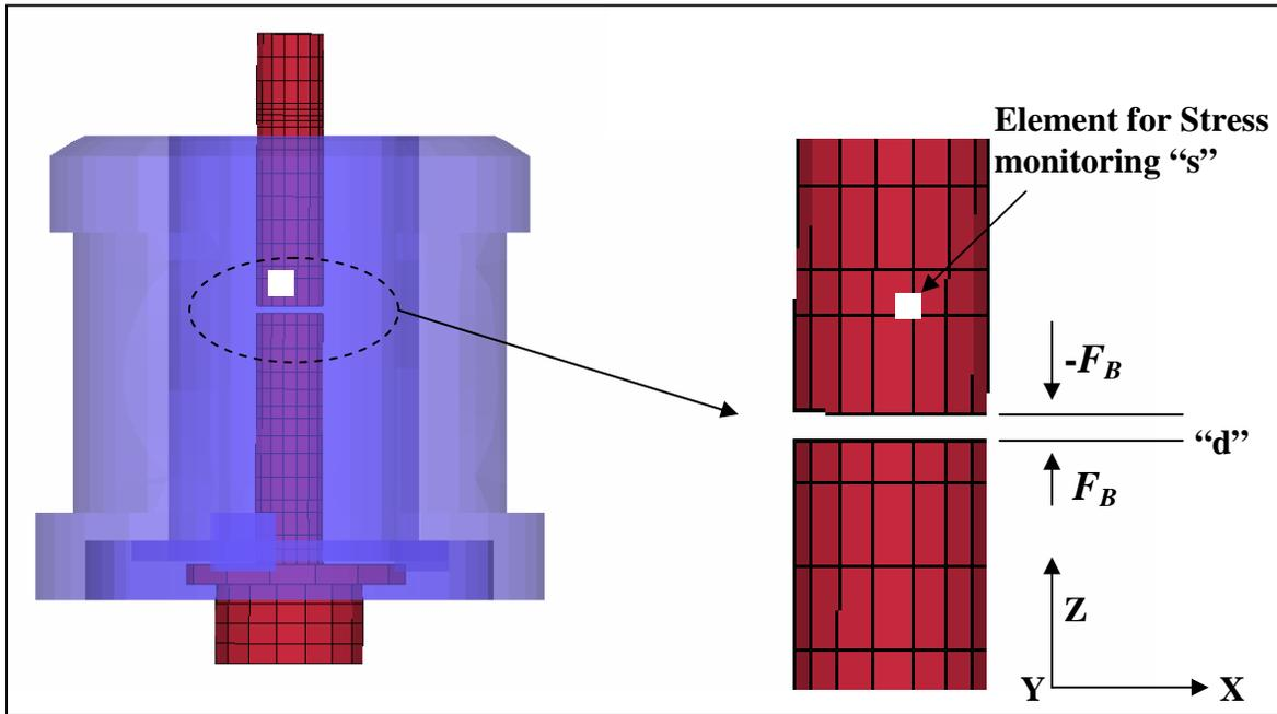
Figure 3. FE (LS-DYNA) model of Pre-Loading for Fastening Core Bolt
