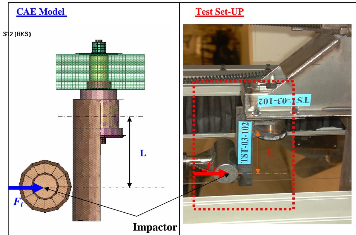
Figure 6. FE (LS-DYNA) model and Validation Test Set-UP for Mount Impact Loading
