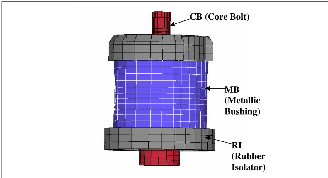
Figure 2. FE (LS-DYNA) model of a sample Flexible Mount
