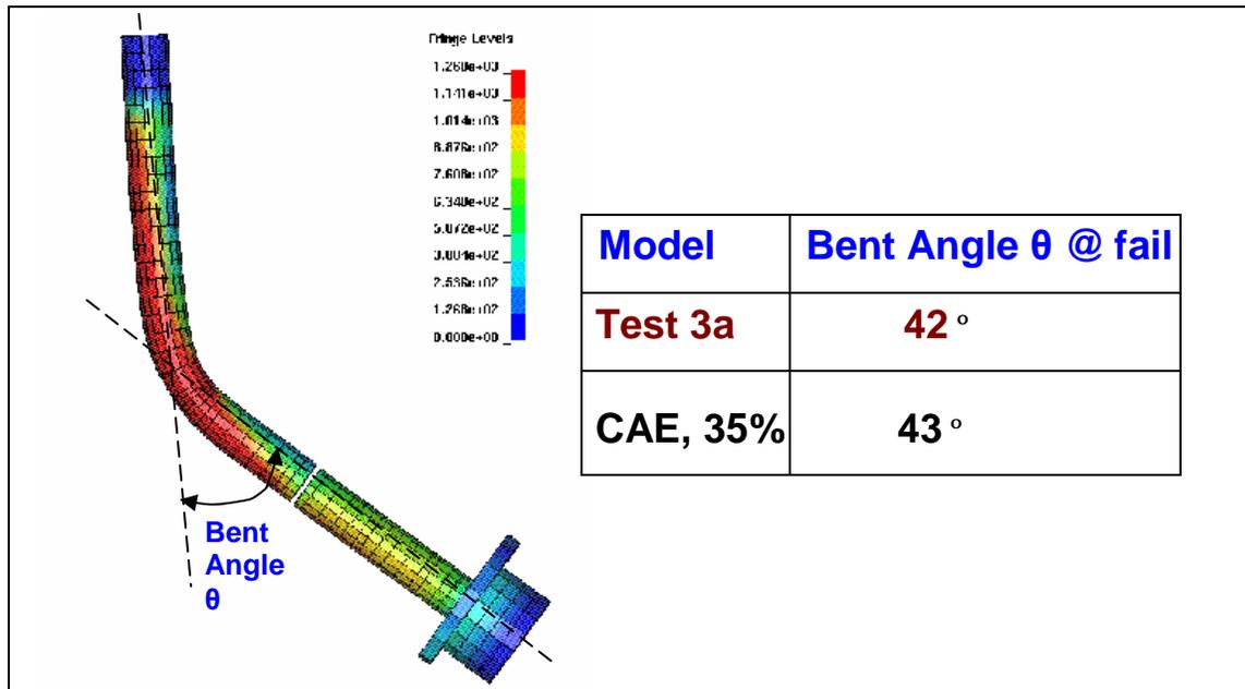
Figure 11. Bent Angle Comparison at Bolt Separation for Test vs. CAE Aluminum Isolator
