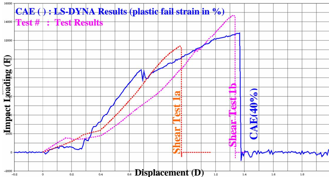
Figure 12. F-D Curves for Test and CAE analysis for Rubber Isolator under Purely Shear Loading
