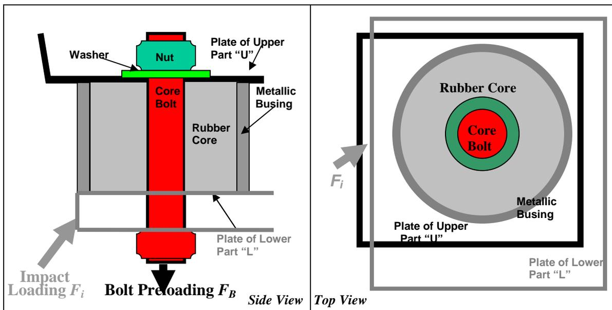
Figure 1 Schematic section view of a sample vehicle rubber mount model
