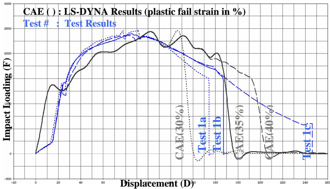
Figure 7. F-D Curves for Test and CAE analysis for Soft(S) Rubber Mount
