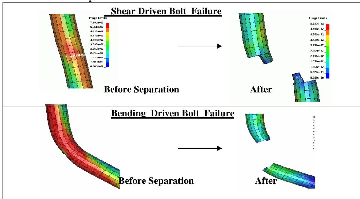
Figure 13. Bolt Separation Modes Comparison for Shear Vs. Bending Loading Cases
