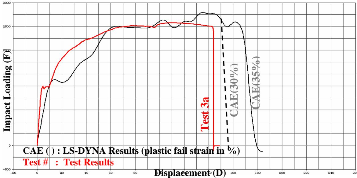
Figure 10. F-D Curves for Test and CAE analysis for Aluminum Isolator
