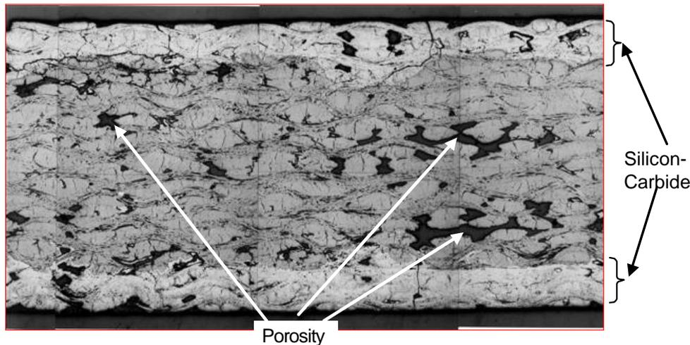
Figure 1. Micro-graph cross-section of 19-ply RCC material.
