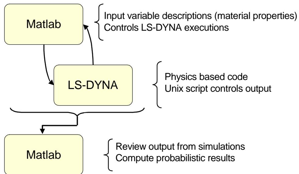
Figure 5. Schematic of probabilistic analysis.
