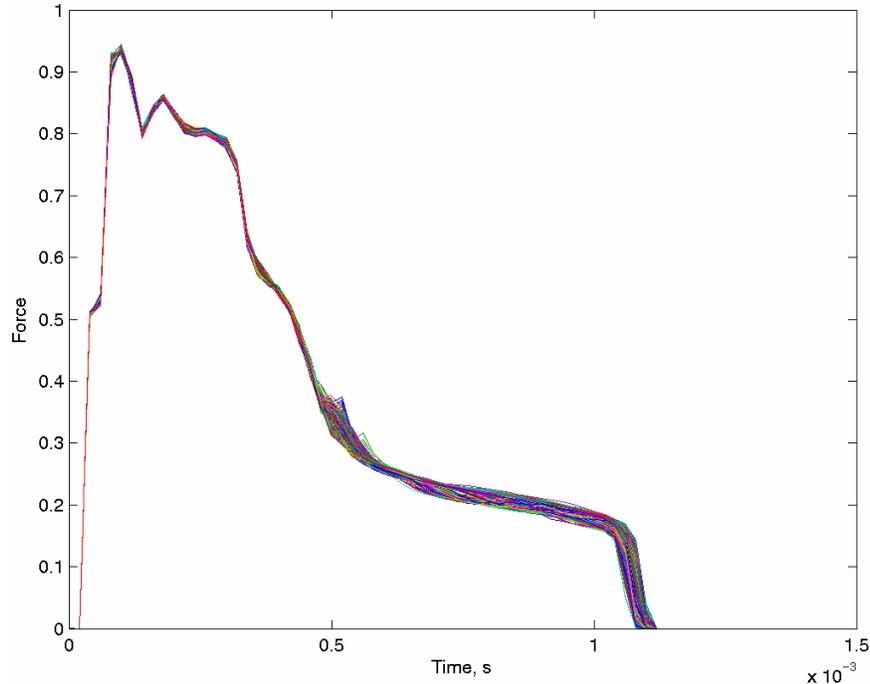
Figure 8. Contact force (non-dimensional) for 500 Monte Carlo simulations.
