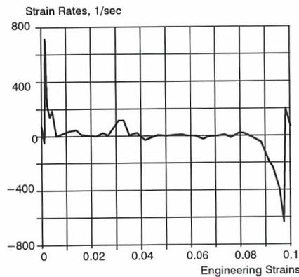
Fig. 3. Strain rates versus engineering strains from the Fig.1 loading stage records.
