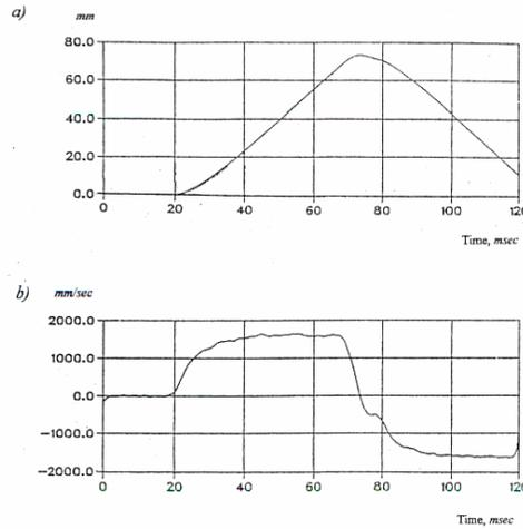
Fig. 1. Records from low velocity impact tests: a) displacements, b) velocity.
