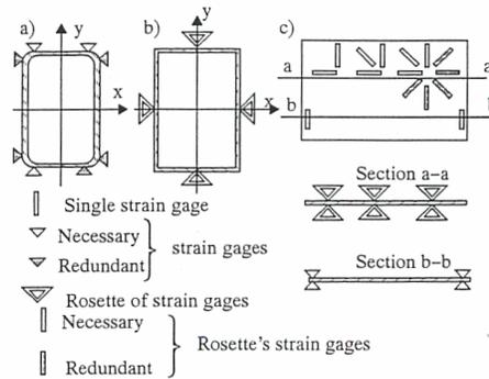
Fig. 4 Examples of strain gage locations on a vehicle structure: a) gages in cross sections b) rosettes in cross sections, c) rosettes and gages on panels
