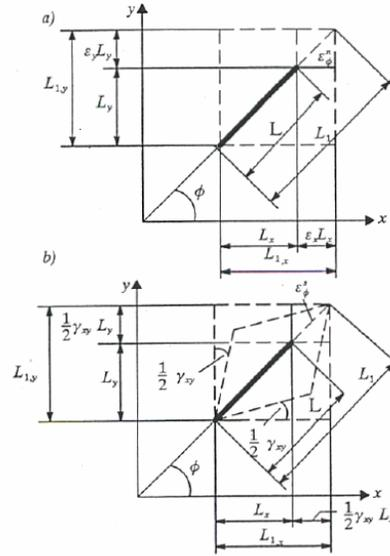
Fig. 5. Strain gage longitudinal deformations from a structure surface normal and shear deformations.
