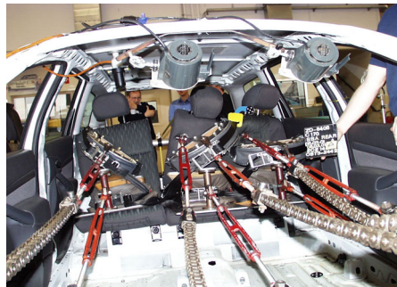
Figure 16. Seat Structure after ECE 14 Test
