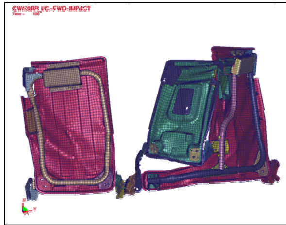
Figure 11. Deformed Structure (OEM’s forward Impact load case)
