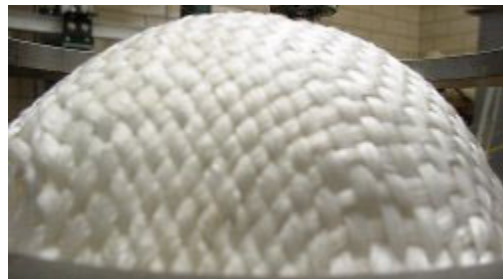
Figure 1. The main mode of deformation when a woven fabric is stamped is shear
