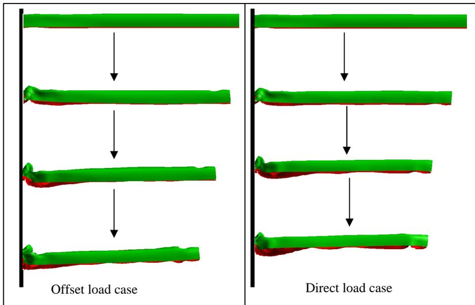
Figure 6. These progressive short-column buckling modes of crush depicted are inherently robust against off-axis dynamic load cases. Energy is absorbed primarily through plastic deformation of the material and friction due to surface contact through the progressive accordion-like deformation. These accordion-like deformation modes help to maximize the plastic material deformation and folding contact during off-axis and direct axis crash scenarios.
