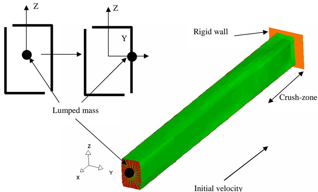
Figure 1. Two open “L” shaped surfaces are welded together to create a closed surface. The rail structure is crushed into the rigid wall due to the initial velocity of the system. The lumped mass is positioned at the end of the structure at various “Y” offsets to create the direct and the offset cases. The peak crush force is measured at the rigid wall while the internal energy is measured in the crush-zone.
