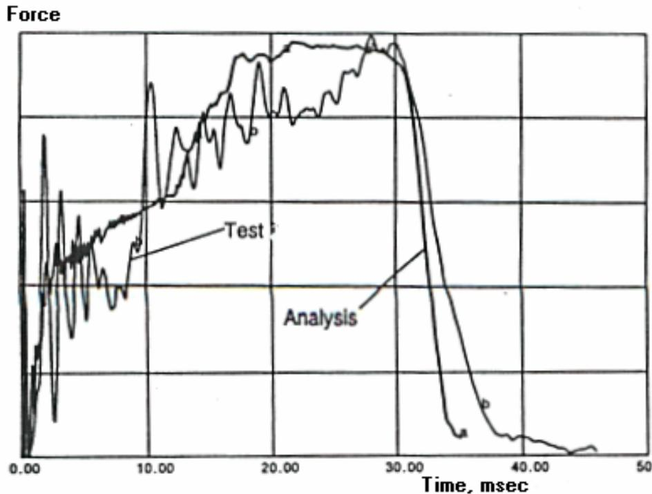
Fig.8. Analysis: Curve from the MDB-to-Skateboard impact test simulation using the static Test curve from Fig. 6.Test: MDB-to-Skateboard impact test curve.
