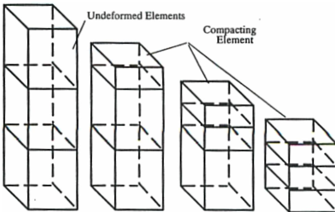
Fig.10. Progressive (localized) brick elements deformation using stress-strain curve with negative slopes, Fig. 6.
