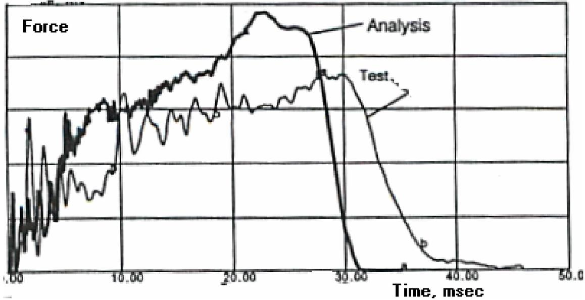
Fig.7. Analysis: Curve from the MDB-to-Skateboard impact test simulation using the Drop Silo test curve from Fig. 6.Test: MDB-to-Skateboard impact test curve.
