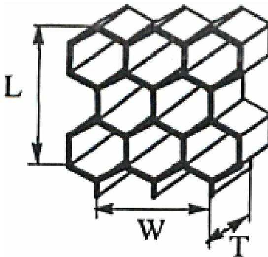
Fig.1. Aluminum honeycombs cellular structure.
