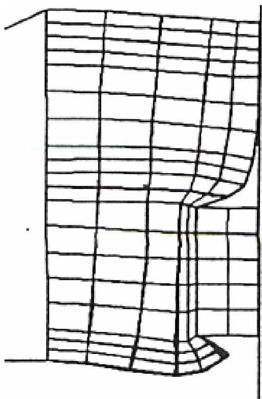
Fig.11. Localized honeycomb brick elements deformation in the MDB.
