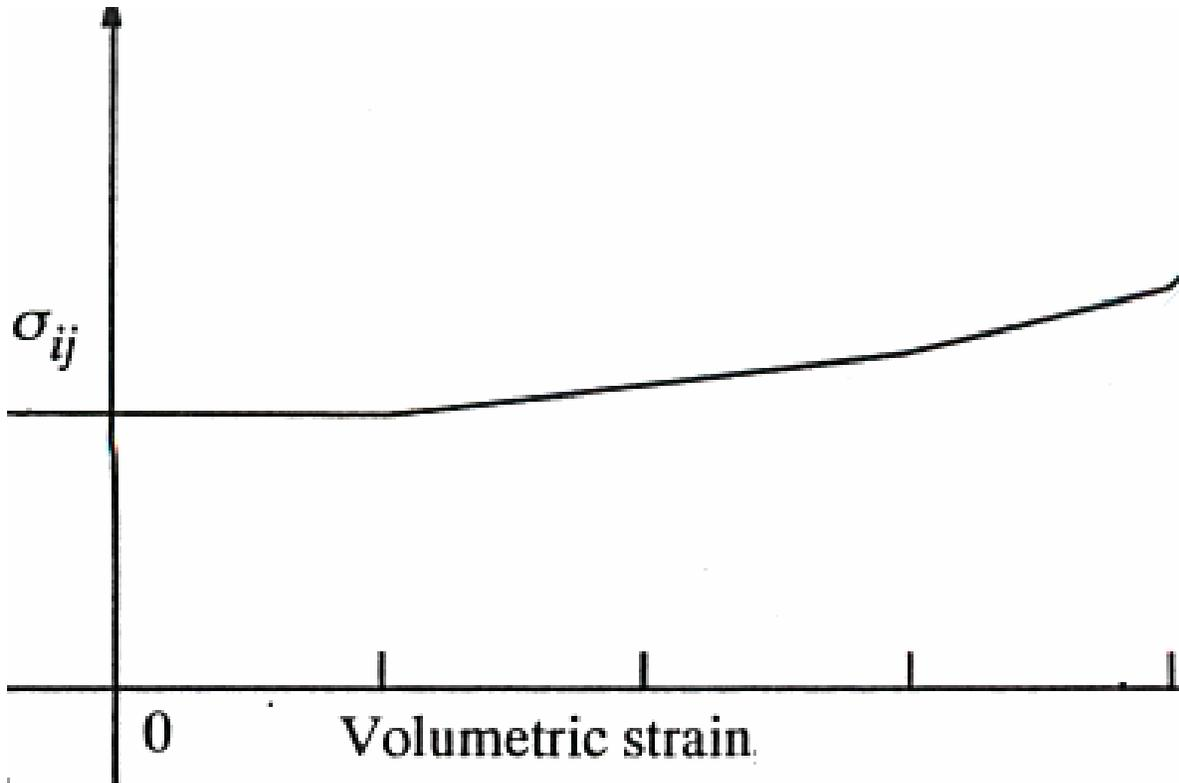
Fig.4. MAT-26 stress-strain input curve.
