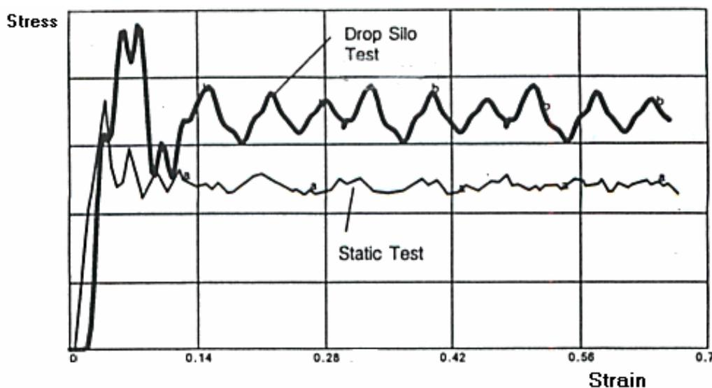
Fig.6. Aluminum honeycomb impact and static test curves.
