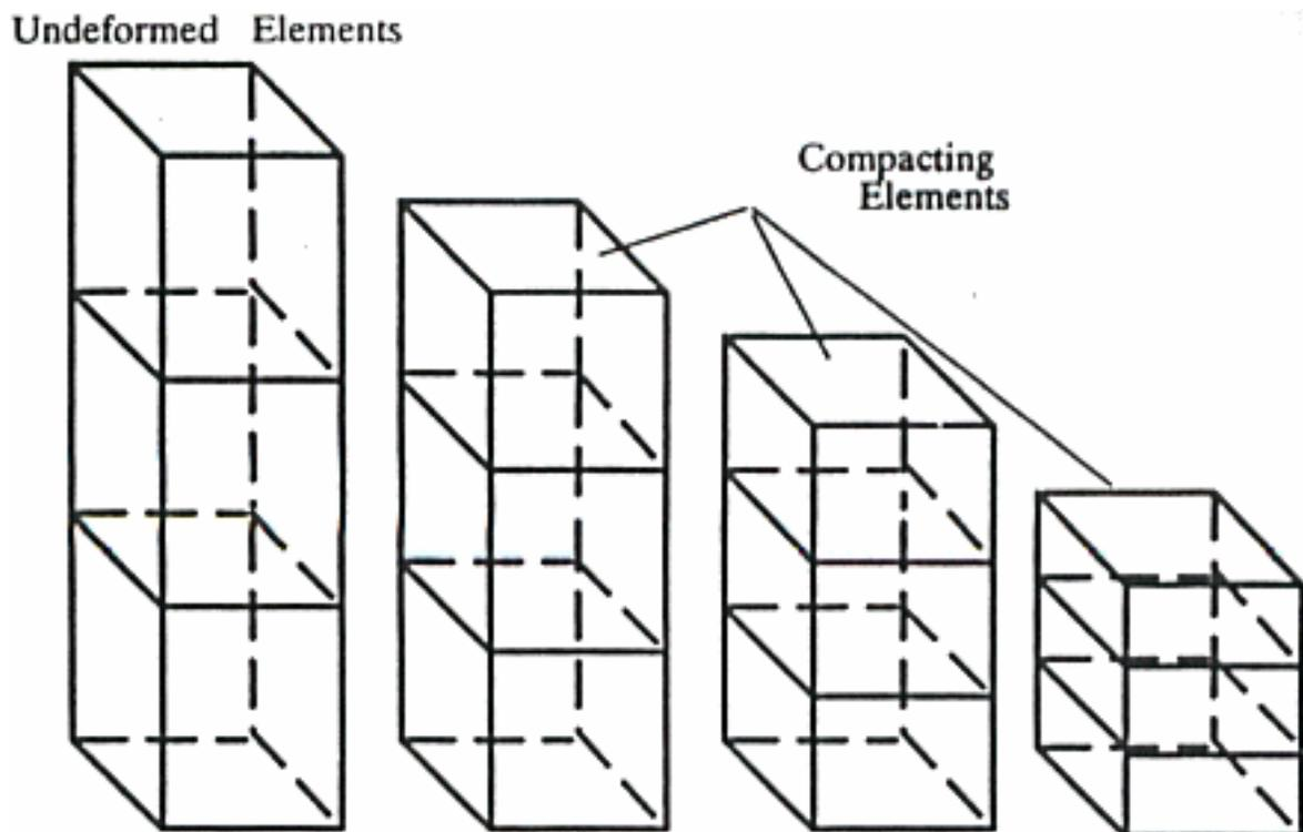
Fig.9. Simultaneous brick element deformation using all positive slopes of stress-strain curve, Fig. 4.
