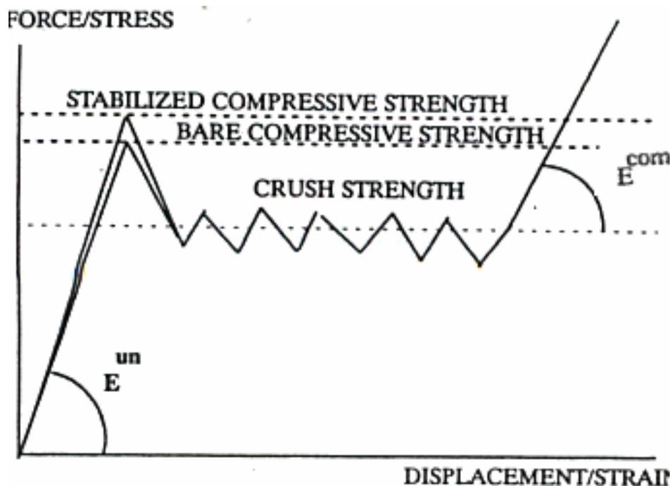
Fig.2. Honeycomb material properties.
