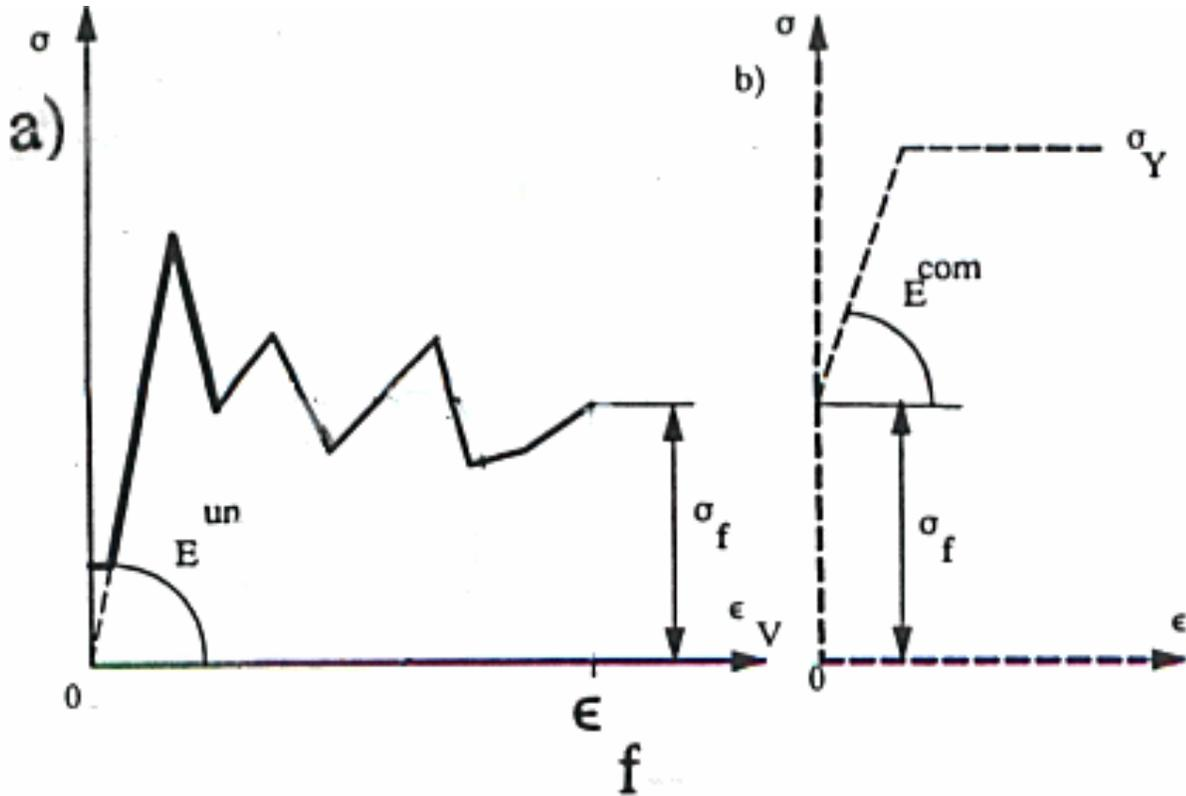
Fig.3. MAT-26 phases: a) not compacted, b) compacted.
