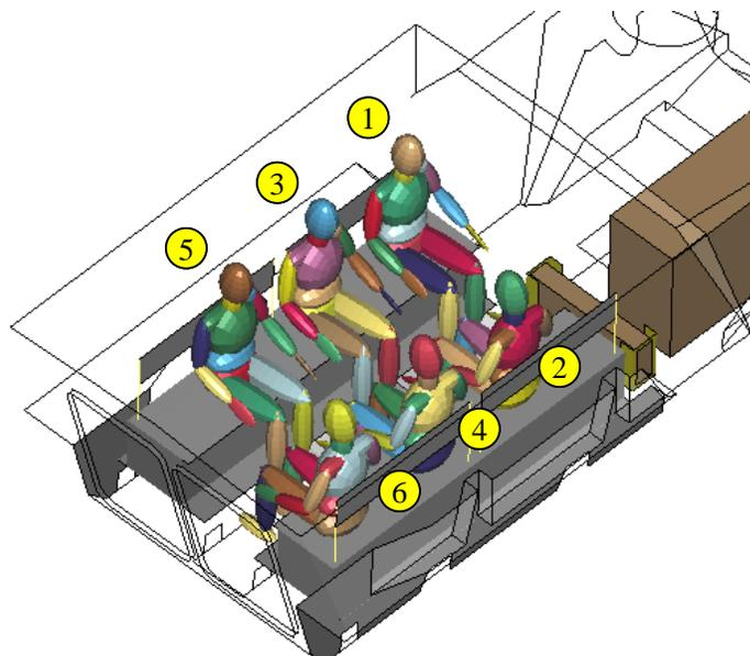
Figure 3. Position of GEBOD dummies inside the vehicle model.
