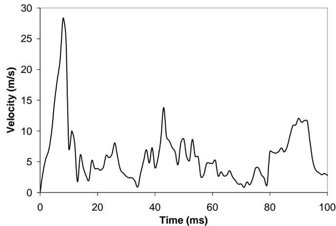
Figure 7. Predicted velocity history of the floor under the feet of GEBOD #5.
