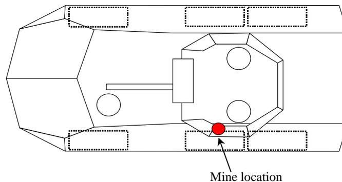
Figure 4. Position of mine relative to vehicle.
