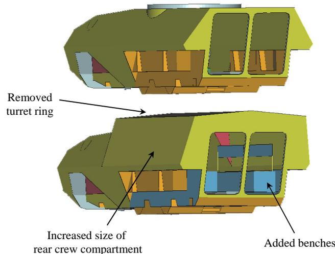
Figure 1. Modification of baseline Cougar model to include rear crew compartment of the LAV-III and seating.
