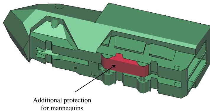
Figure 2. Protection added to baseline vehicle to prevent damage to Hybrid IIIs caused by hull rupture during tests.
