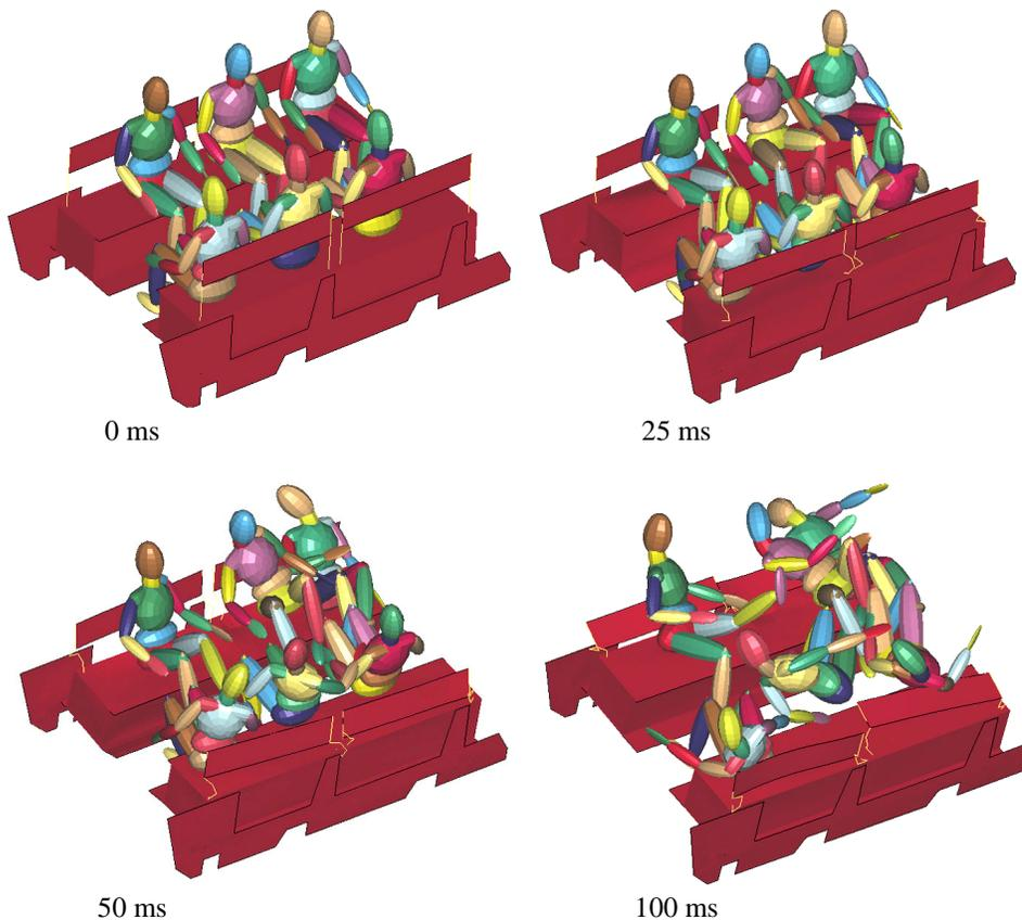
Figure 5. Sequence of GEBOD reactions to the detonation of a 6-kg C-4 mine surrogate under the left centre wheel viewed from the side opposite the mine location (vehicle faces to the right). The vehicle hull has been removed for clarity.
