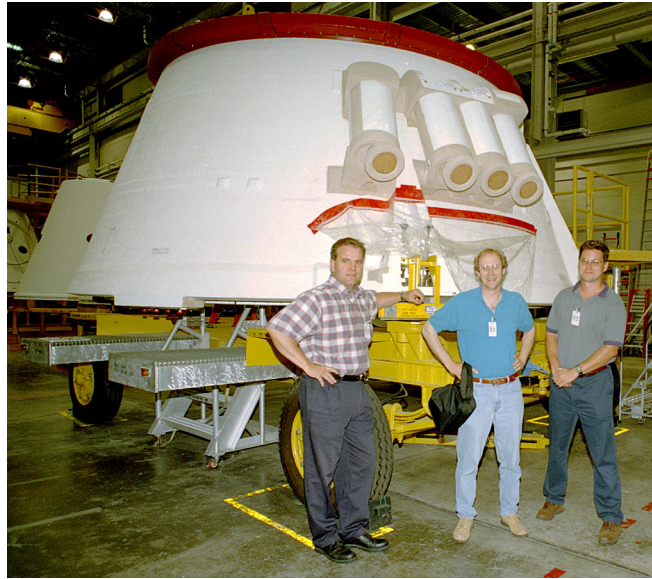
Figure 3. Aft Skirt in NASA Assembly Facility Awaiting Integration to SRB
