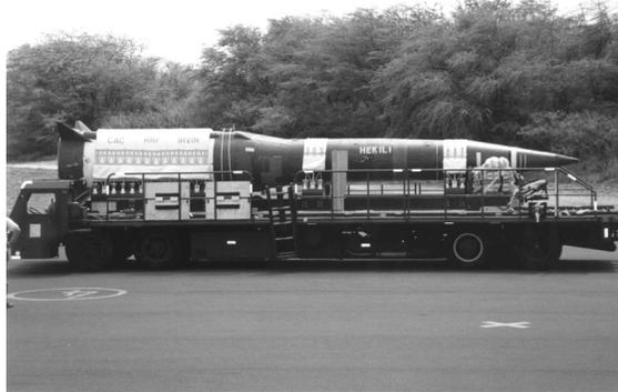
Figure 2. An Example of a Fabric Blanket Constraining a Missile
